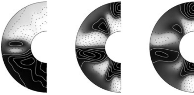
Figure 7. Radial components of the first three dipolar eigenmodes \mathbf{b}^i , i = 1 \dots 3 of the time-averaged dynamo operator for model 2. The corresponding growth rates are \lambda_1 = -3.87 , \lambda_2 = -34.83 and \lambda_3 = -42.45 in units of \eta/L^2 . Note the huge drop in growth rates after \lambda_1 .
