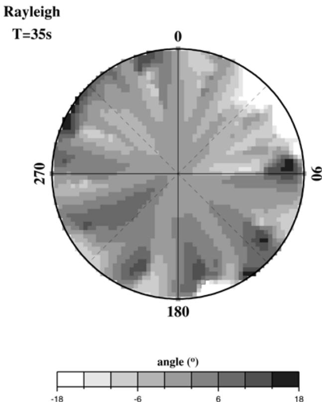
**Figure 7.** Results of the estimation of the angular deviation of the incident Rayleigh wave from the great circle using the linear perturbation theory (Woodhouse & Wong 1986) for a large number of possible source locations. The model used is that of Ekström *et al.* (1997) for a 35 s period Rayleigh wave. The greyscale indicates the sign and value of the deviation calculated at the station.
