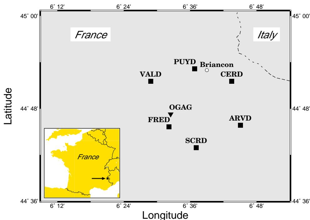
**Figure 1.** Map of the locations of the six broad-band stations installed in the French Alps for the GéoFrance3D programme from August to December 1996. The temporary mini-array (black squares) describes a circle with a diameter of approximately 25 km. The black triangle shows the permanent station OGAG of the Observatory of Grenoble.
