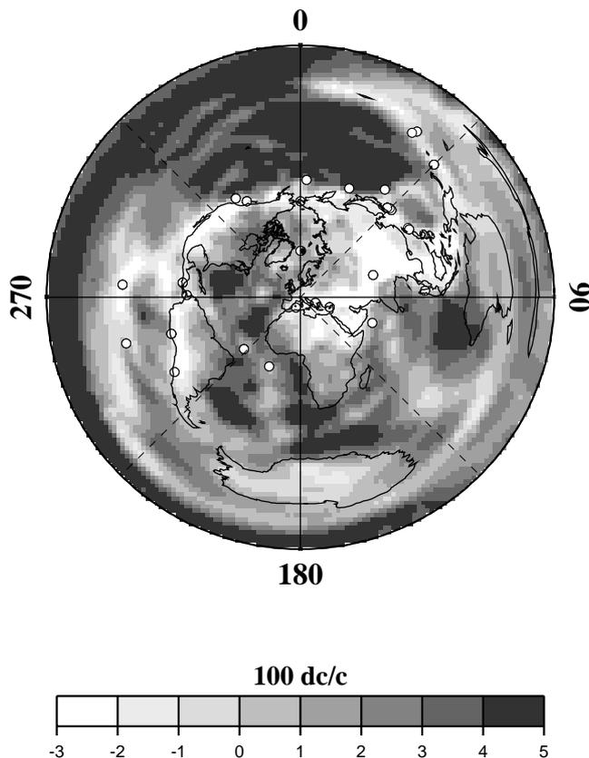
**Figure 2.** Locations of the 36 events (white circles) used for the array analysis in a polar representation. The greyscale in the background shows the phase velocity model (Ekström *et al.* 1997) for the 35 s period Rayleigh wave. The representation is centred on the centre of the array GEOF (see Fig. 1) and the distance from the centre gives the epicentral distance between 0 and 180° directly.
