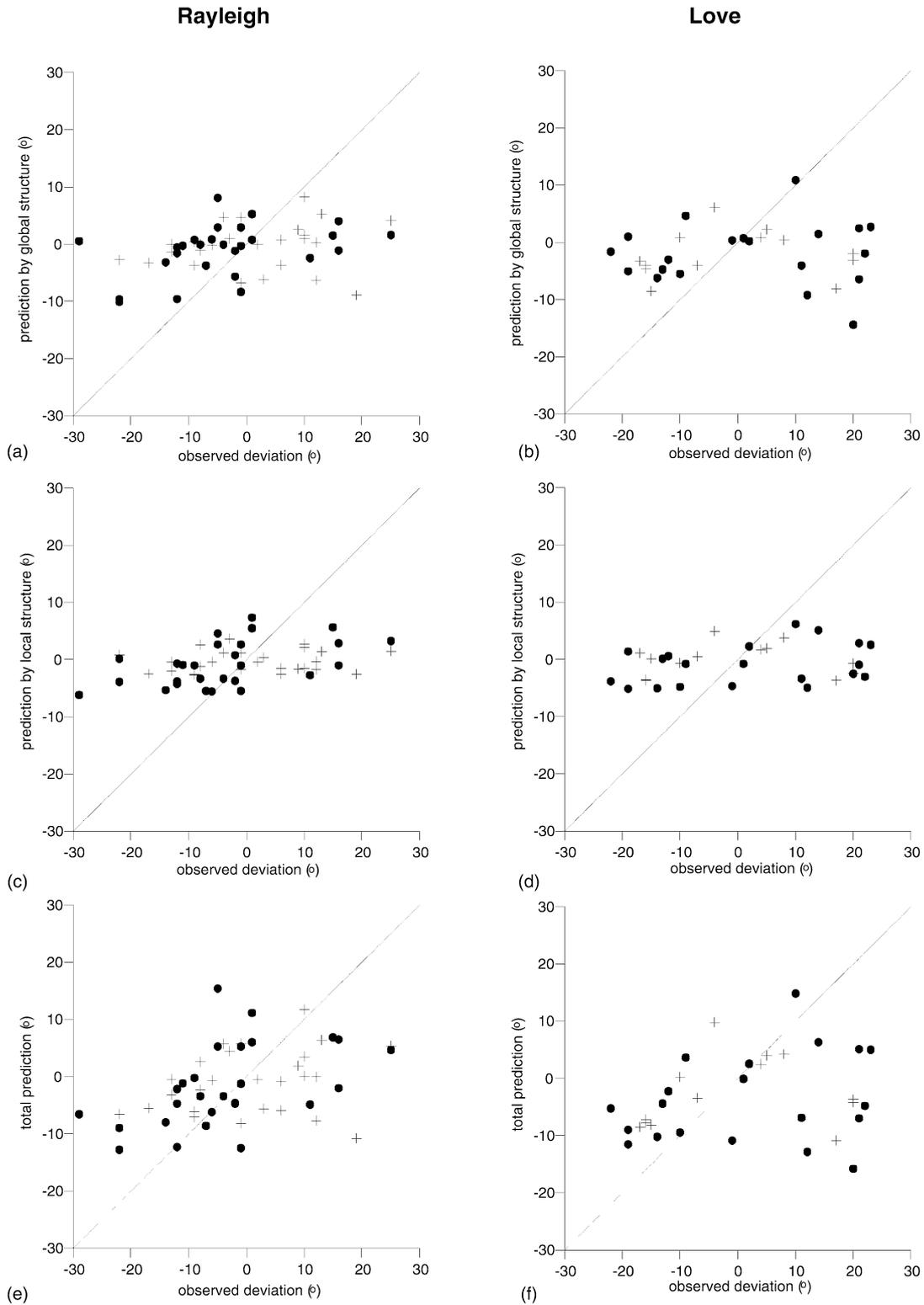
**Figure 10.** Results of the deviations calculated for Rayleigh (left column) and Love waves (right column) as a function of the observed deviations. The solid circles are for  $T = 35$  s and the crosses for  $T = 50$  s. (a), (b) Predictions calculated in global models. (c), (d) Predictions calculated in the local structure. (e), (f) Total predictions as the superposition of the global and local structures.
