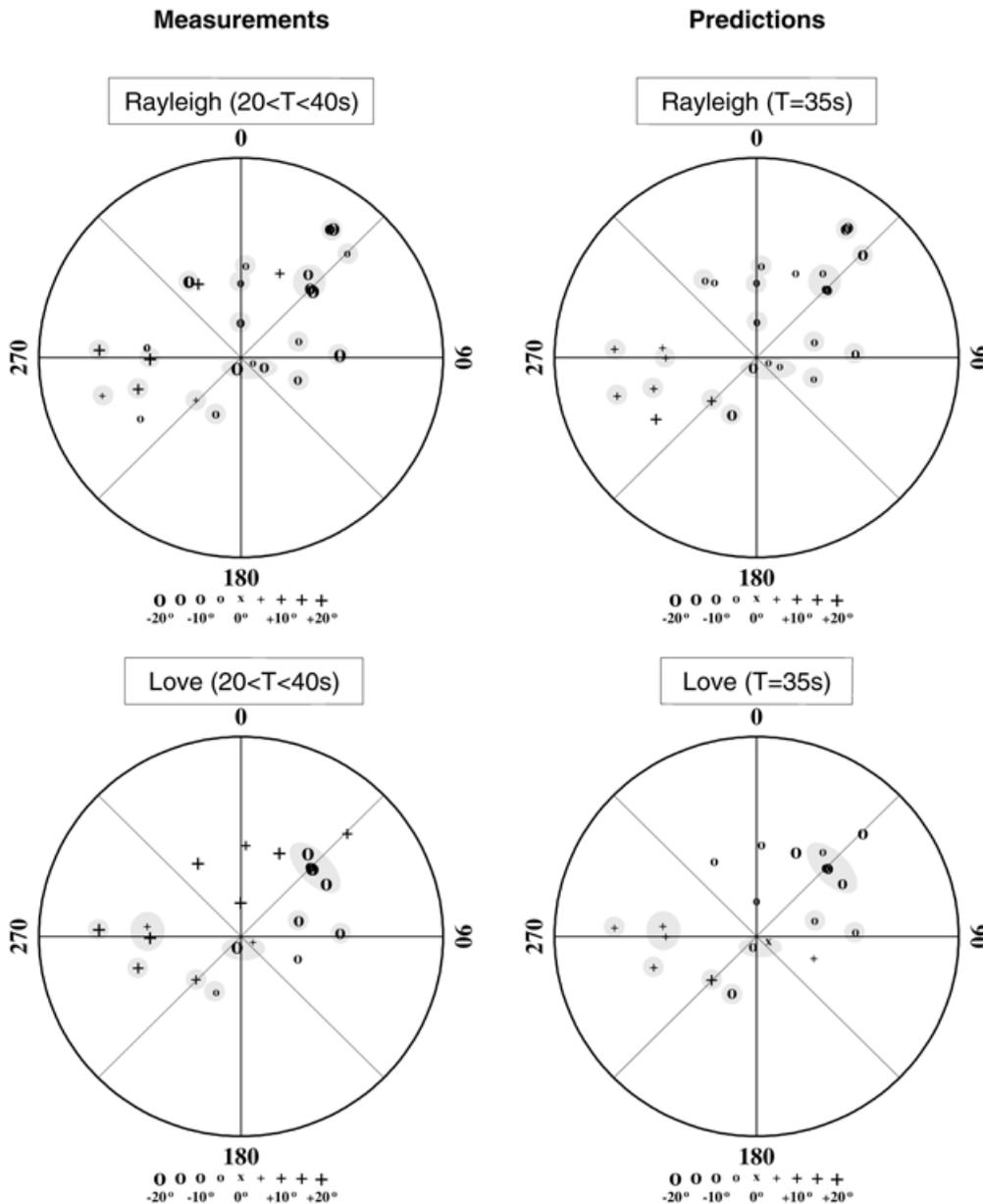
**Figure 11.** Comparison between measured (left column) and predicted (right column) deviations at a station located in the French Alps. Top: Rayleigh waves; bottom: Love waves. Measurements are for signals between 20 and 40 s, and predictions are for 35 s period. Grey shading corresponds to points with a reasonable fit between observations and predictions.
