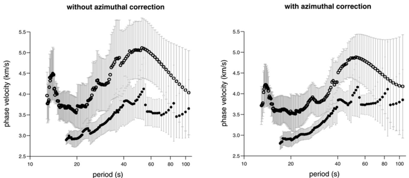
**Figure 12.** Phase velocities presented as a function of the period. The left-hand figure shows the phase velocities obtained without the azimuth correction, and the righthand figure shows the phase velocities for incident waves corrected for the off-great-circle deviations. Open and solid circles are respectively for Love and Rayleigh waves. Grey bars show the standard deviation of the phase velocity measurements.
