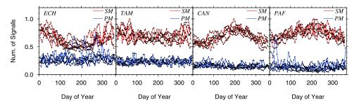
**Figure 6.** Number of elliptical polarized signals in a vertical plane as function of day of the year. Plotted are the normalized moving averages obtained from 50% overlapping 10 day data windows. The results for the 7 years are plotted on top of each other. Frequency bands are 0.05–0.09 Hz and 0.1–0.14 Hz for the primary (PM, blue lines) and secondary (SM, red lines) microseisms, respectively.
