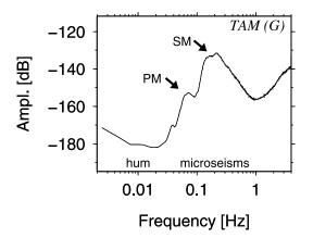
**Figure 1.** Vertical component power spectrum for 1 year of noise recorded at station Tamanrasset, Algeria (TAM). "Hum" and "microseism" mark the frequency ranges where they occur. The hum is not observed in Figure 1. The primary and secondary microseismic peaks are marked by PM and SM, respectively. Other noise sources occur in all frequency bands.
