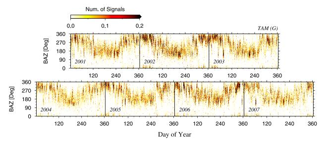
**Figure 8.** Number of elliptical polarized signals in a vertical plane as function of back azimuth (BAZ) and day of the year. The frequency band is 0.09-0.15 Hz, and the nonoverlapping bins have a size of 1 day  $\times$  3°. The number of counted signals is normalized to 1.
