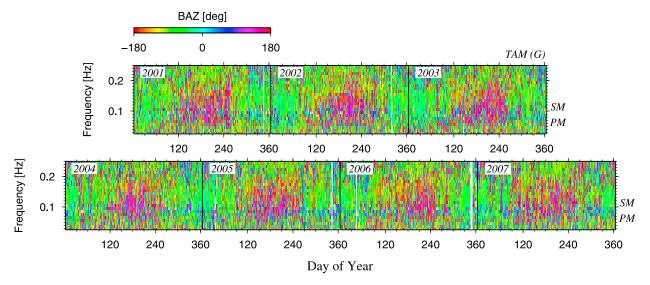
**Figure 9.** Most often measured back azimuth (BAZ) as function of time and frequency at station TAM. The seasonal dependence of BAZ is visible. BAZ points toward the south during Northern Hemisphere summer due to increased ocean storm activity in the Southern Hemisphere.
