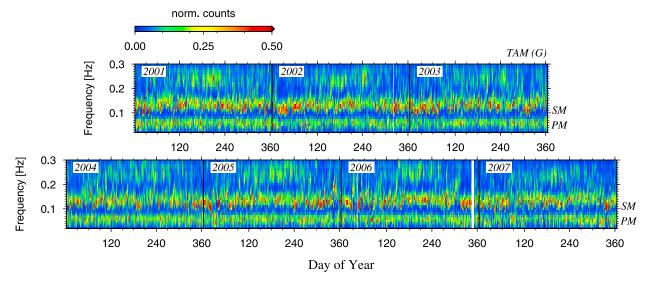
**Figure 5.** Polarization spectra as function of time and frequency for station TAM. The red colors correspond to the maximum number of polarized signals which are normalized to 1. The color scale is saturated at dark red above 0.5 to increase the visibility of smaller amplitude features. The PM and SM are omnipresent and visible as horizontal red bands at about 0.07 and 0.14 Hz, respectively. White is used whenever there is a day with no signal with degree of polarization above our threshold.
