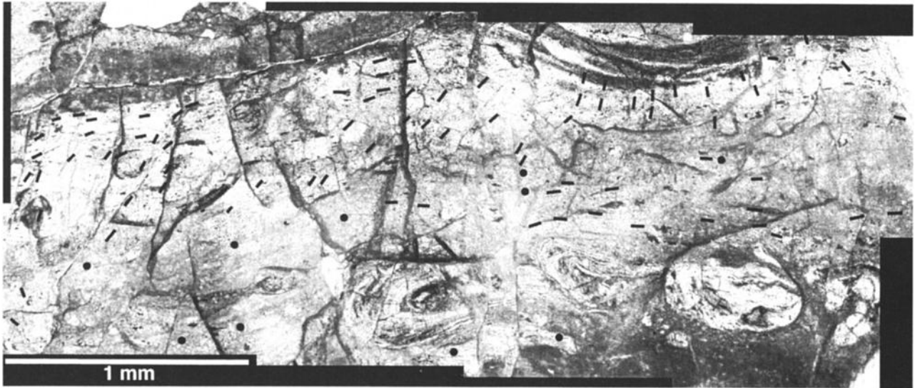
Figure 3. Microphotograph showing the layering and disrupted folds of an older pseudotachylyte layer embedded in a younger one. The long axes of the ellipsoidal fluid inclusions are indicated by the short, black lines.
