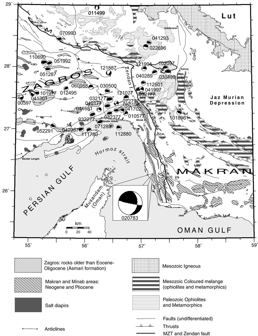
**Figure 2.** Structural map of the Zagros-Makran transition zone, modified after the 1:2,500,000 geological map of Iran. The Zendan fault trace is modified after this work (see hereafter). “Beach balls” represent Harvard CMT fault mechanisms for the period 1976–2002 (the date is mentioned mmddyy), the only one clearly related to the Minab-Zendan fault zone is enlarged. For clarity, rocks younger than Oligocene have not been drawn in the Zagros.
