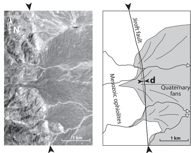
**Figure 14.** SPOT satellite image of site J01 and interpretative sketch (alluvial fans are shaded). Solid arrows show the Jiroft fault trace and “d” represents its deviation through alluvial fans, indicating the fault plane dips to the west.
