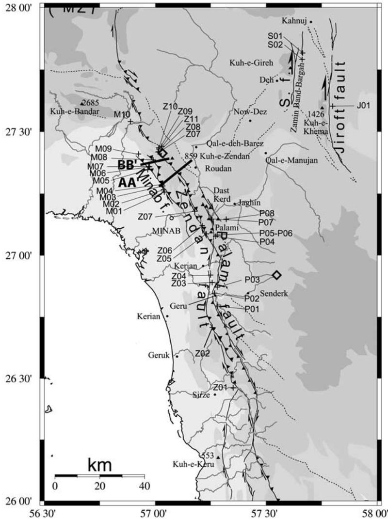
**Figure 6.** Map of the active faults, showing their motion, and location of cross sections of Figure 4; site striation measurements are indicated. Diamonds are locations of folds studied by *Delaunay et al.* [2002]. Note that the N160°E trending segments are transpressive while north trending ones are pure strike-slip faults. See Figure 5 for general legend.
