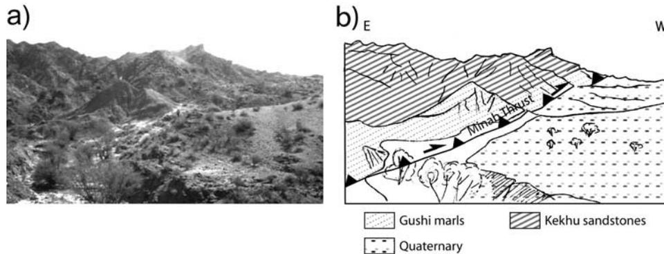
**Figure 7.** (a) South facing view of site M04 (Demchehr). (b) Interpretative drawing showing the trace of the Minab thrust. Quaternary corresponds to a terrace contemporaneous with the high pediment  $Qt_1$ .
