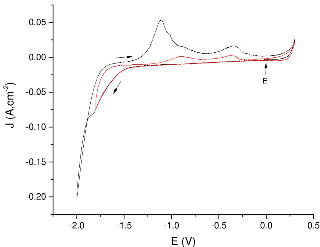
Fig. 2- Cyclic voltammogram at a Pt electrode in  $\text{Li}_2\text{CO}_3\text{-K}_2\text{CO}_3$  under 100 mol%  $\text{CO}_2$  at 650 °C. Scan rate  $100 \text{ mV s}^{-1}$ . Reverse potential at -1.8 V and -2 V vs  $\text{Ag}^+/\text{Ag}$ .
