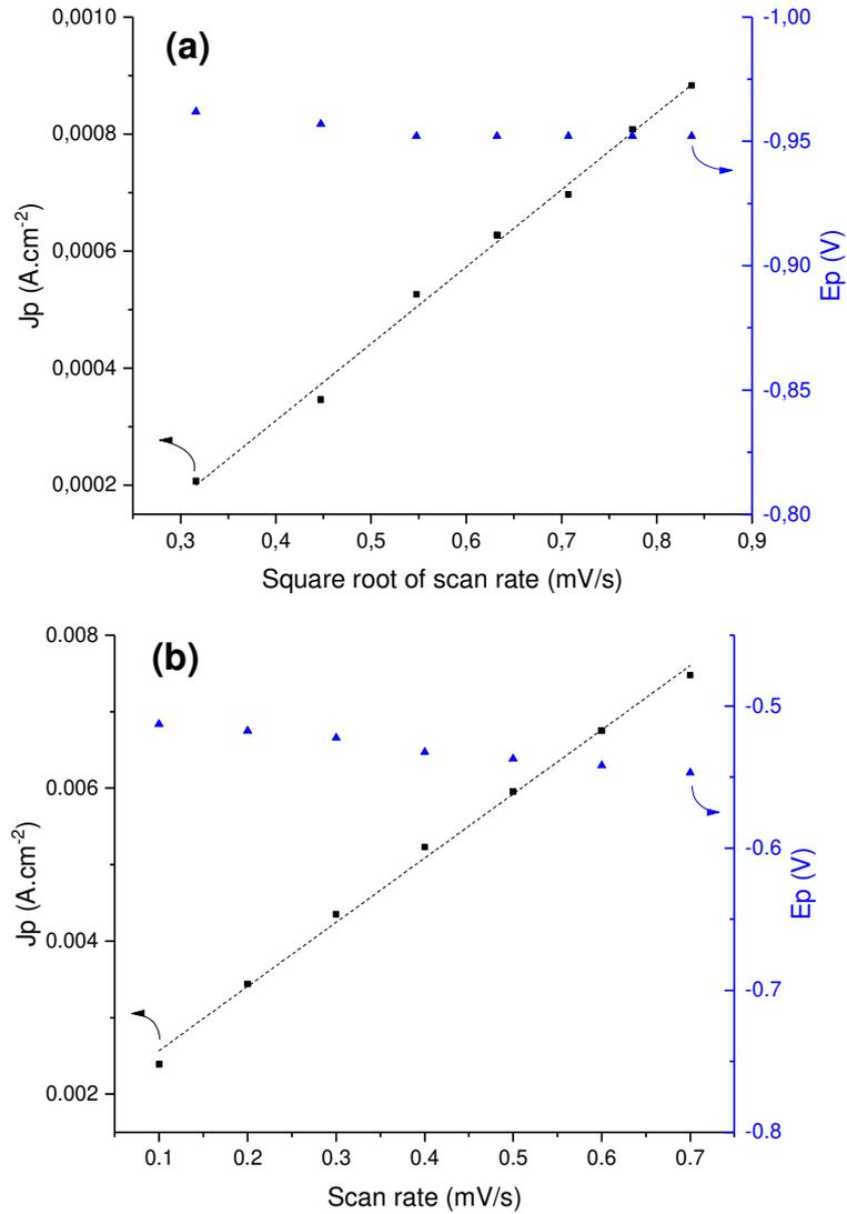
Fig. 4- Evolution of both oxidation peak potentials and currents with scan rate, with a the first (around -1 V vs Ag<sup>+</sup>/Ag) and b the second peak (around -0.5 V vs Ag<sup>+</sup>/Ag).
