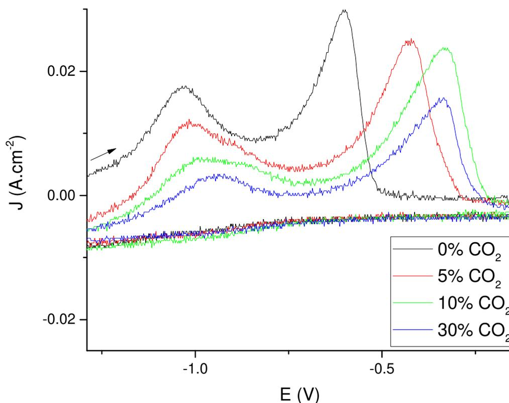
*Fig. 5- Cyclic voltammogram reverse scans on a Pt electrode at 100 mV/s under 70 mol% H<sub>2</sub>O and various amounts of CO<sub>2</sub>.*
