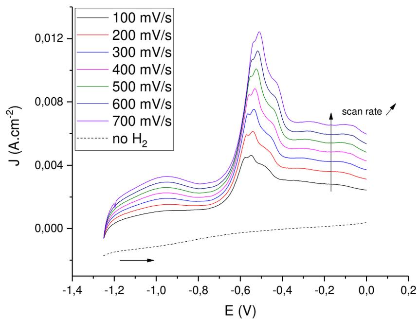
Fig. 3- LSV on a Pt electrode at various scan rates under 64 mol% H<sub>2</sub>/20 mol % H<sub>2</sub>O/16 mol % Ar.
