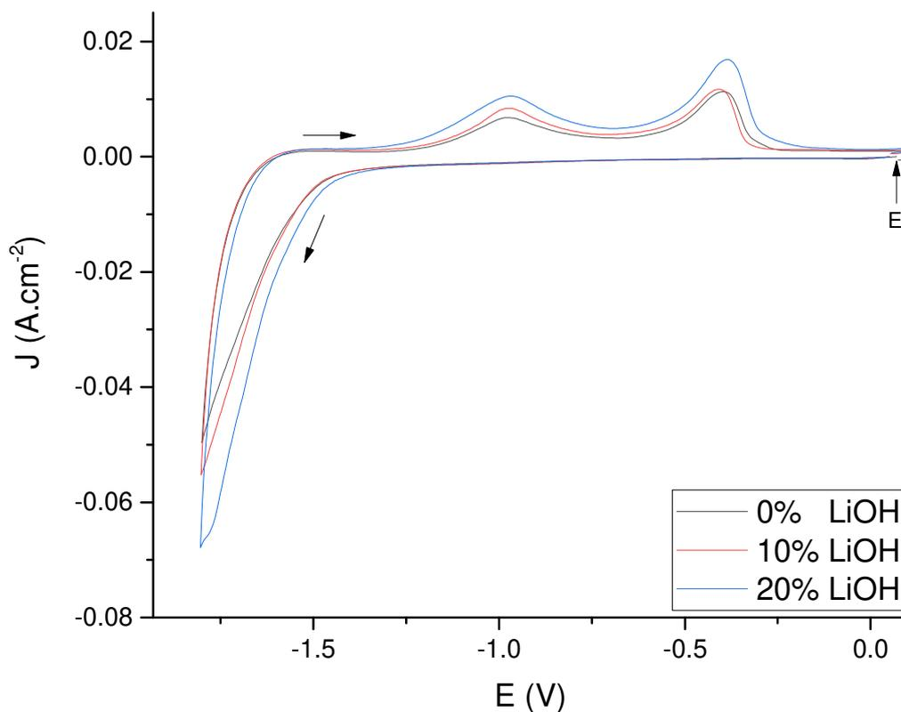
Fig. 7- Cyclic voltammograms on a Pt electrode at 100 mV/s under 70 mol% H<sub>2</sub>O/15 mol% CO<sub>2</sub>.
