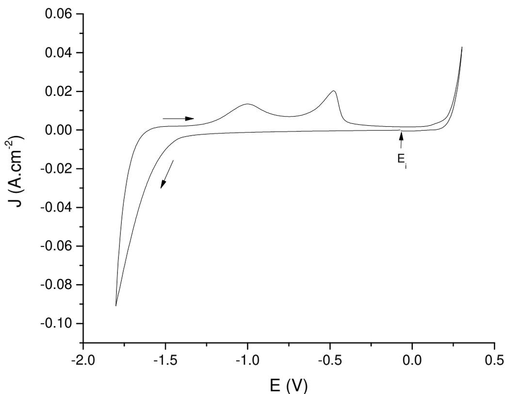
Fig. 1- Cyclic voltammogram at a Pt electrode in Li<sub>2</sub>CO<sub>3</sub>-K<sub>2</sub>CO<sub>3</sub> under 70 mol% H<sub>2</sub>O/30 mol% Ar at 650 °C. Scan rate 100 mV s<sup>-1</sup>.
