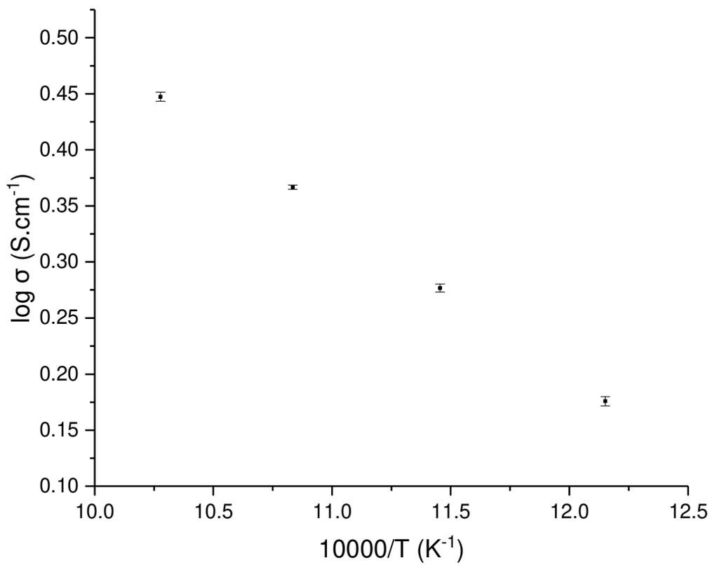
*Fig. 10- Example of an Arrhenius plot for 50 mol% of added LiOH.*
