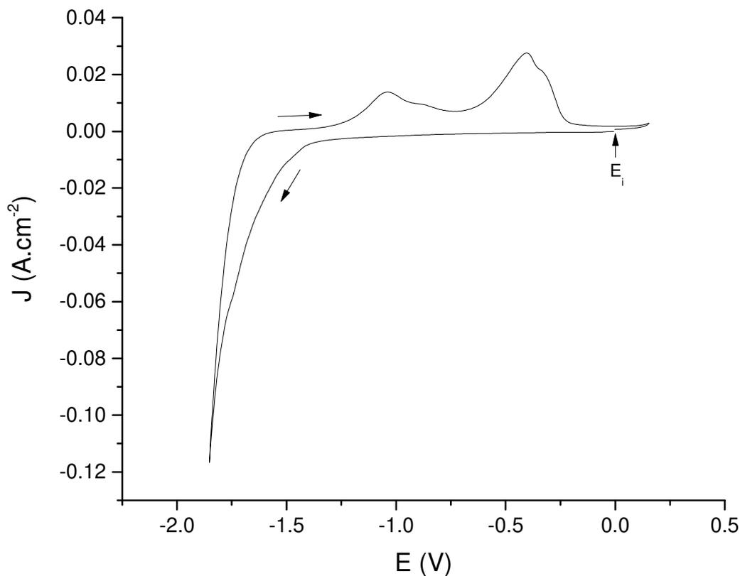
*Fig. 8- Cyclic voltammogram on a Pt electrode at 100 mV/s under 100 mol% CO<sub>2</sub> right after 40 mol% LiOH addition.*
