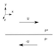
Fig. A.1. Configuration of the stratified flow.
