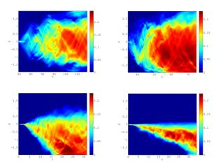
**Fig. A.3.** Mixing due to the KHI. From left to right, top to bottom:  $\alpha = 0, 0.5, 0.9, 0.99$ .
