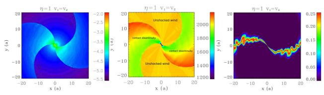
**Fig. 4.** Small-scale simulation: density, velocity, and mixing for a simulation with identical winds ( $\eta = 1$ ,  $\beta = 1$ ). The density is given in g cm<sup>-2</sup>, the velocity is in km s<sup>-1</sup> and the mixing of the winds is a dimensionless variable. The length scale is the binary separation a.
