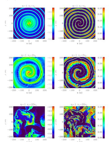
**Fig. 7.** Large-scale simulation: density (*left column*) and mixing (*right column*) for simulations with  $\{\eta = 1, \beta = 1, 2, 20\}$  (from top to bottom) in the large boxes. The length scale is the binary separation a. The mixing of the winds is a dimensionless variable.
