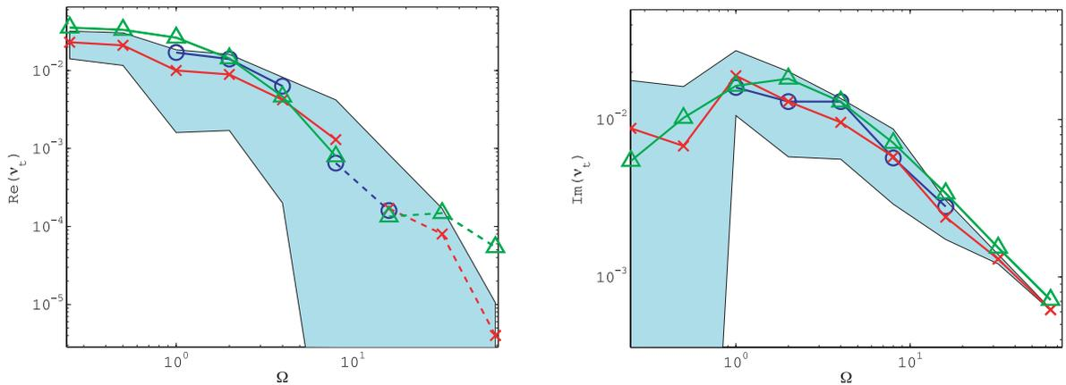
**Figure 4.** Turbulent viscosity of spanwise convection, versus the angular oscillation frequency in units of  $|N|$ . The numerical measurements are shown in blue (open circles;  $S = 0.1$ ) and red (crosses;  $S = 0.05$ ) and the best fit of the closure model (61) is shown in green (triangles). Negative values are connected by a dashed line. Uncertainties due to turbulent noise are shown as a shaded region.
