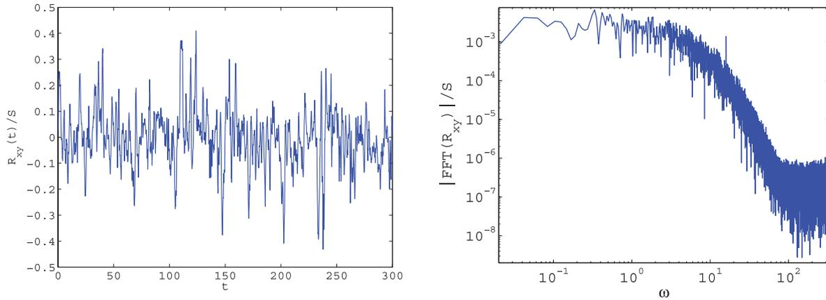
**Figure 2.** Time history of the Reynolds stress (left) and Fourier transform of the Reynolds stress (right) with an oscillatory shear of frequency  $\Omega = 16$  and amplitude  $S = 0.1$ . The periodic signal cannot be seen in the time series. The Fourier transform exhibits a peak at the excitation frequency  $\omega = \Omega$ .
