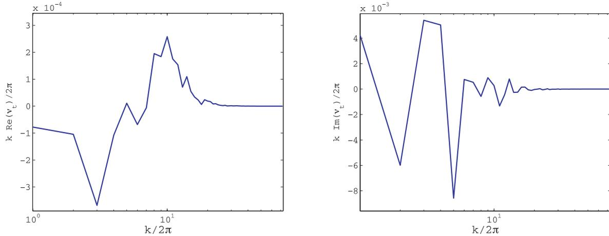
**Figure 5.** Spatial spectrum of the turbulent viscosity for the simulation of spanwise convection with  $\Omega = 16$  and  $S = 0.1$ . The real part has two components: a negative contribution from large scales and a positive contribution from smaller scale ( $k/2\pi \sim 10$ ).
