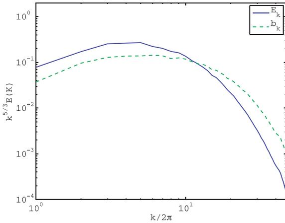
**Figure 1.** Simulation snapshot of thermal fluctuations (top) and energy spectra (bottom) at  $Ra = 4 \times 10^6$  in the case without any shear. We show the kinetic energy spectrum ( $E_k$ ) and the temperature fluctuation spectrum ( $b_k$ ).
