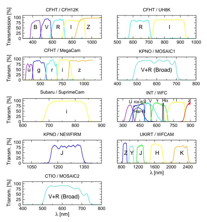
Fig. 2. Transmission of the various filters used in this study. In the z-band, the sensitivity is limited by the CCD quantum efficiency, which typically drops at 900  $\sim$  1000 nm.
