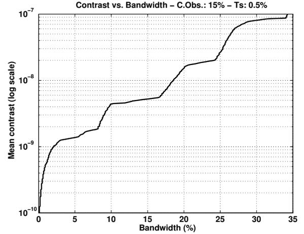
**Fig. 11.** Mean contrast as a function of the bandwidth (in %) for a charge 4 VC, and an aperture with 15% central obscuration and 0.5% thick spiders. The contrast is measured between the IWA and the OWA of the coronagraph, inside an annulus.
