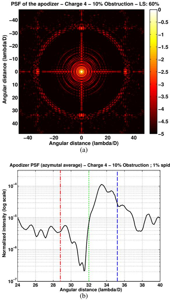
**Fig. 10.** 2D **a)** and azimuthal average **b)** of the PSF of the optimal apodizer designed for a 10% central obscuration, 1% thick spiders, and a charge 4 vortex. In the azimuthal average, the red dot-dashed line denotes the highest spatial frequency captured by the mask at  $\lambda = 1.1\lambda_0$ , the blue dashed line does the same  $\lambda = 0.9\lambda_0$ , and the dotted green line does it at  $\lambda = \lambda_0$ .
