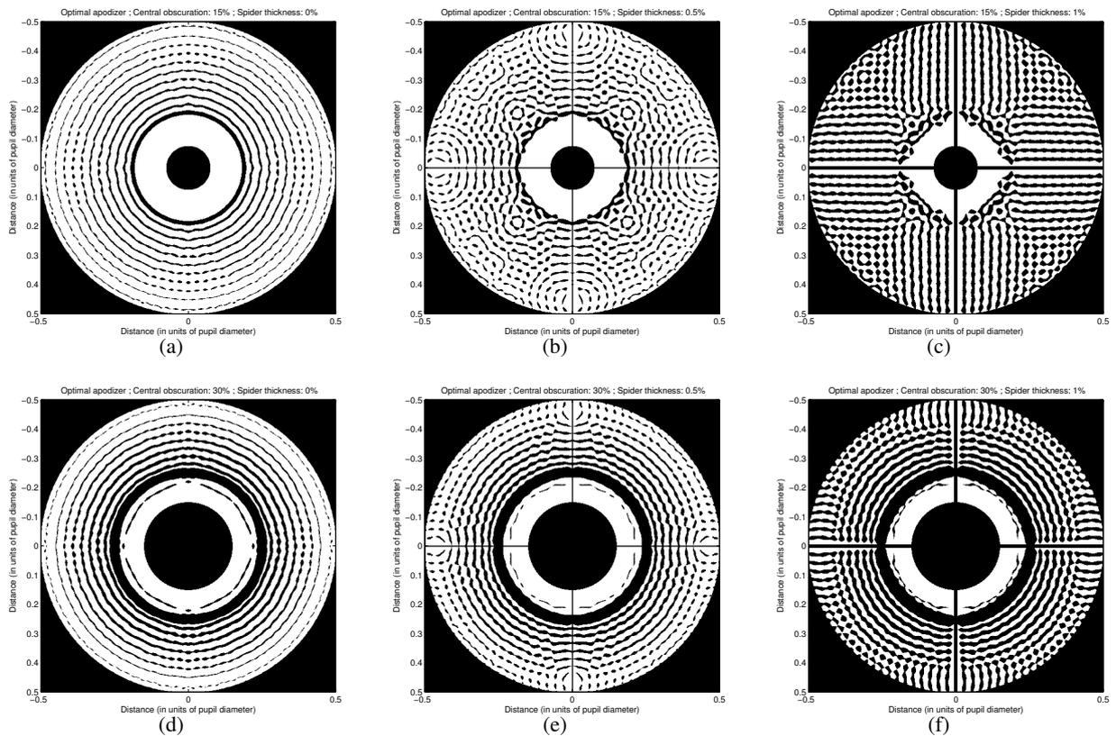
**Fig. 5.** Apodizers giving the highest system throughput for a charge 4 VC used with a 10% (*top*) and a 30% (*bottom*) central obscuration, and three spider thicknesses: 0, 0.5, and 1% (from *left to right*).
