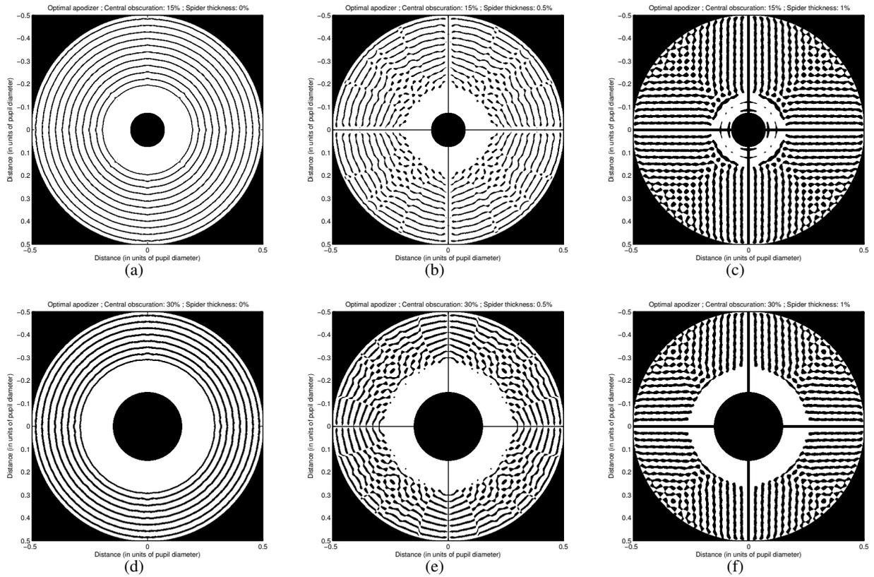
**Fig. 4.** Apodizers giving the highest system throughput for a charge 2 VC used with a 10% (*top*) and a 30% (*bottom*) central obscuration, and three spider thicknesses: 0, 0.5, and 1% (from *left to right*).
