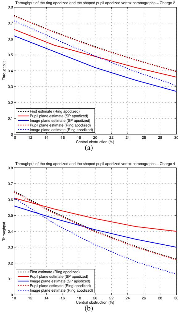
**Fig. 3.** Comparison of the throughputs estimates of the ring apodized VC (dotted lines) and the shaped pupil apodized VC (solid lines) for topological charges 2 and 4. Different measures of the throughput are illustrated. Pupil plane estimates are showed in red, while image plane estimates are showed in blue. The dotted black line represents the throughputs given in Mawet et al. (2013b).
