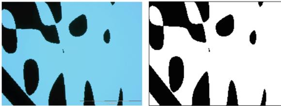
**Fig. 12.** Comparison of the theoretical and actual transmissions of a portion of a 2D shaped pupil manufactured for the Subaru telescope. *Left:* microscope photography of the mask. *Right:* corresponding desired profile. Each pixel has a  $10\ \mu\text{m}$  size.
