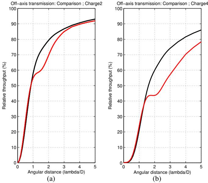
**Fig. 6.** Comparison of the relative off-axis transmission of the VC (black line) and an AVC (red line) designed for a  $CO_A = 20\%$  obscured aperture with  $t_S = 0.5\%$  spiders. The comparison is made for **a)** a charge 2 vortex and **b)** a charge 4 vortex. The transmissions are normalized with respect to the coronagraph throughput  $T_{\max}$ .
