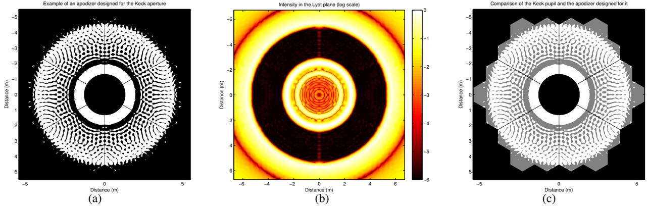
**Fig. 2.** Example of a design for the Keck telescope, a charge 4 vortex coronagraph, and a circular Lyot stop: **a)** apodizer transmission; **b)** intensity in the Lyot plane (log scale); and **c)** comparison of the Keck aperture and the apodizer. In the last figure the apodizer is represented in white, while the Keck aperture is represented in gray (wherever the apodizer transmission is zero).
