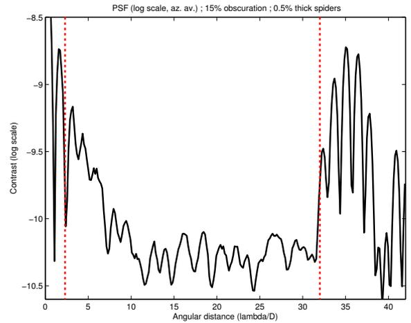
**Fig. 9.** Coronagraphic PSF (azymutal average) for the apodized vortex designed for a 15% centrally obscured aperture and 0.5% thick spiders. The intensity is displayed on a log scale. Angular distances are given in units of  $\lambda/D$ .
