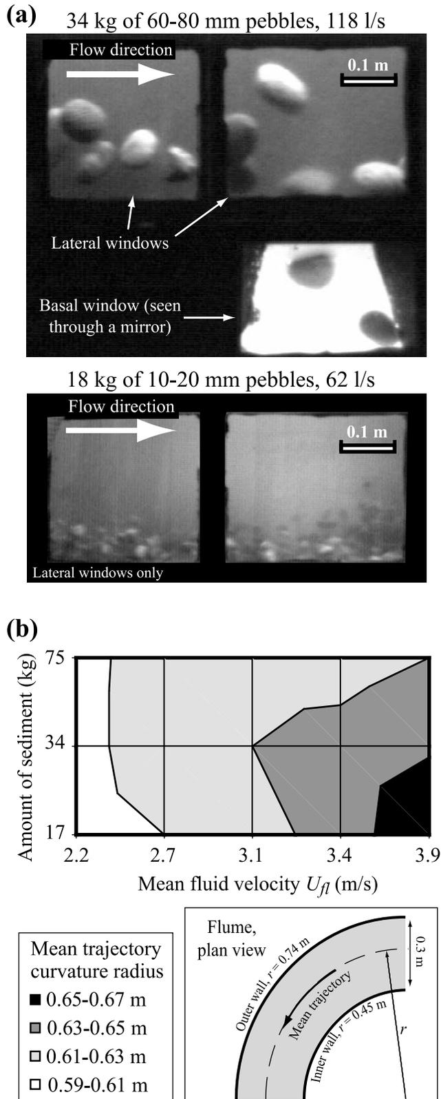
**Figure 2.** (a) Snapshots of movies recorded with a high speed camera to track the trajectories of pebbles in saltation during experiments with (top) 34 kg of 60–80 mm pebbles and an input discharge of 118 l/s and (bottom) 18 kg of 10–20 mm pebbles and an input discharge of 62 l/s. (b) Mean trajectory curvature radius as a function of fluid velocity and sediment amount for the 60–80 mm pebbles. Trajectories with large curvature radius are observed for high velocity and low sediment amount.
