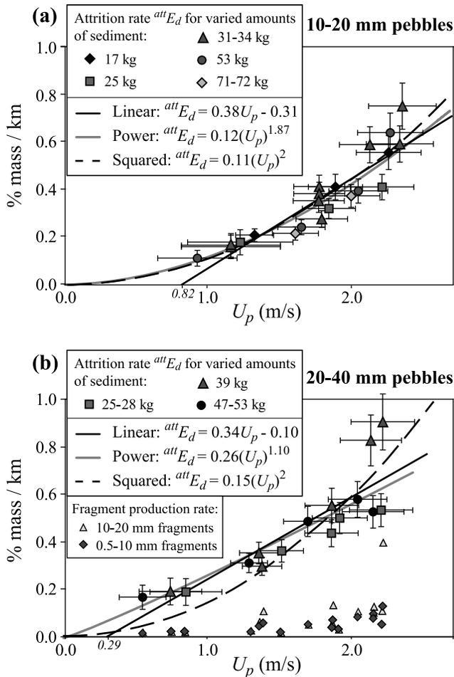
**Figure 5.** Attrition rate  $^{att}E_d$  (in percent mass per km) as a function of pebble velocity  $U_p$  for different amounts of sediment, for experiments carried out with (a) 10–20 mm pebbles and (b) 20–40 mm pebbles. Regression curves and their equations are shown for 3 models: linear, power, and squared. In Figure 5b, the rate of fragment production  $^{fr}E_d$  (in percent mass per km) is also represented.
