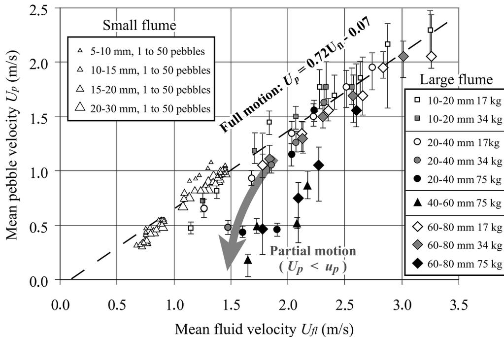
**Figure 3.** Mean pebble velocity during a round trip as a function of mean water velocity in the flumes. Both small and large flume data describe a linear relationship at full motion. For low velocity and/or large amount of sediments, data depart from the trend, because round trips include both motion and resting periods. Particle velocities are obtained using three different methods (see text); average values (data points) and maximum and minimum values (tips of “error” bars) are shown.
