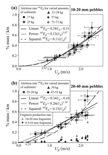
**Figure 5.** Attrition rate  ${}^{att}E_d$  (in percent mass per km) as a function of pebble velocity  $U_p$  for different amounts of sediment, for experiments carried out with (a) 10–20 mm pebbles and (b) 20–40 mm pebbles. Regression curves and their equations are shown for 3 models: linear, power, and squared. In Figure 5b, the rate of fragment production  ${}^{fr}E_d$  (in percent mass per km) is also represented.
