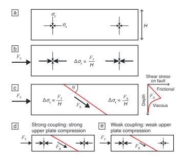
**Figure 6.** Sketch illustrating the concept of plate coupling.  $\sigma_x$  and  $\sigma_z$  are the horizontal stress and vertical stress, respectively.  $F_T$  is a tectonic force laterally applied to a lithosphere of thickness H.  $\Delta \sigma_x$  is the average differential stress resulting from the force  $F_T$ .  $F_S$  is the plate coupling force and, that is, the integrated shear stress along the fault dipping at angle  $\theta$ . See text for details.
