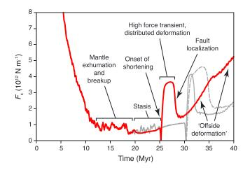
**Figure 9.** Temporal evolution of the horizontal force  $F_X$  applied to extend or shorten the model at a given rate. Red line is for the reference model (20-Myr rifting followed by shortening at a rate of 4 mm/year), gray solid line for alternative model 1 (25-Myr rifting, 4 mm/year shortening), and gray dashed line for alternative model 2 (25-Myr rifting, 2 mm/year shortening).
