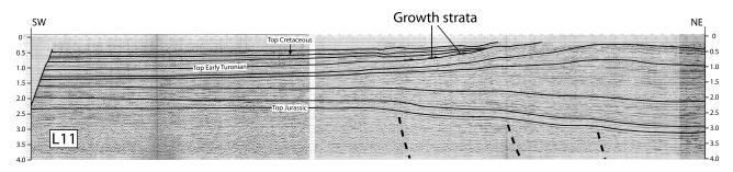
**Figure 7.** Longitudinal seismic section (L11) through the Chotts basin (see location in Figure 1b) showing the western border of the extensional Mesozoic basin and the inversion of the El Fejej graben.
