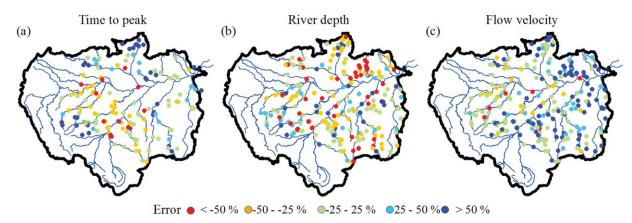
**Figure 4.** Spatial distribution of MAE values for (a) time to peak, (b) river depth, and (c) flow velocity.
