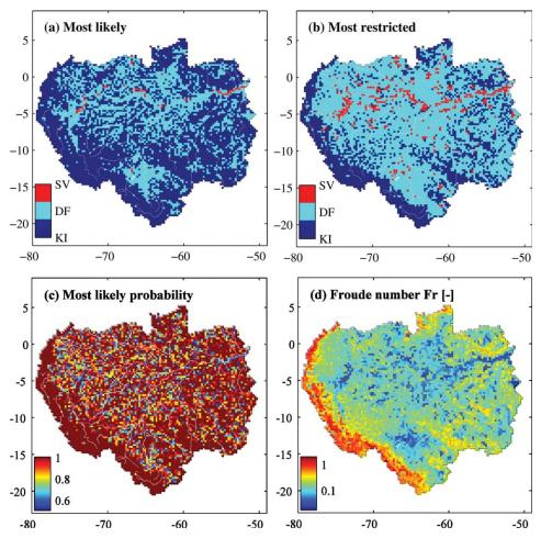
**Figure 5.** (a) Most likely and (b) most restricted flood wave type, (c) frequency of the most probable class and (d) Froude number maps for the Amazon Basin. Flow dynamics are represented by the following flood wave types: kinematic wave (KI), diffusive wave (DF), steady dynamic wave (SD), gravity wave (GV), and full Saint-Venant (SV). The white lines represent the main rivers.
