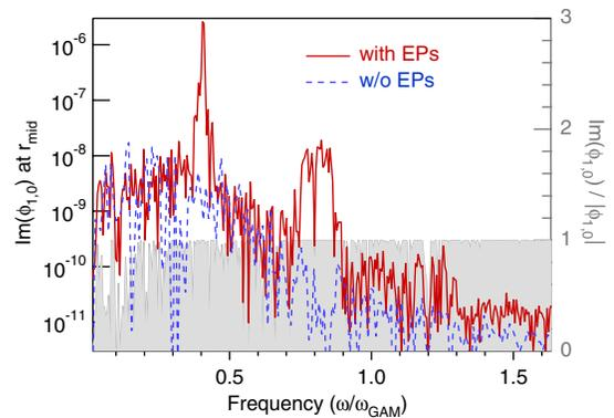
FIG. 3 (color online). Time Fourier transform of the  $\sin\theta$  component of  $\phi_{1,0}$  for both simulations with (solid red line) and without (dotted blue line) EPs. For the simulation with EPs, the imaginary part of  $\phi_{1,0} / |\phi_{1,0}|$  is plotted (shaded region).
