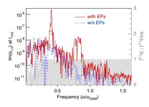
FIG. 3 (color online). Time Fourier transform of the  $\sin\theta$  component of  $\phi_{1,0}$  for both simulations with (solid red line) and without (dotted blue line) EPs. For the simulation with EPs, the imaginary part of  $\phi_{1,0}/|\phi_{1,0}|$  is plotted (shadowed region).
