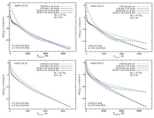
Fig. 22. Disc CO v = 0 rotational population at LTE and at NLTE for the  $R_{\rm in} = 1$  AU models with only the v = 0, v = 1, 2, and v = 1, 2, 3, 4, 5 levels taken into account. All populations have been normalized.
