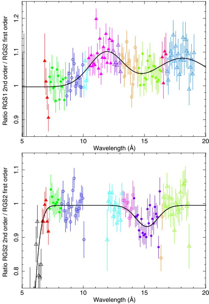
**Fig. 6.** As Fig. 5, but for second-order spectra compared to first-order spectra. Owing to the specific geometry of missing CCDs (CCD7 for RGS1, CCD4 for RGS2) we compare all fluxes to the first order of RGS2. Open symbols: second-order chips 1, 3, 5, 7, 9; filled symbols: second-order chips 2, 4, 6, 8. Triangles: first-order chips 1, 3, 5, 7, 9; circles: first-order chips 2, 6, 8.
