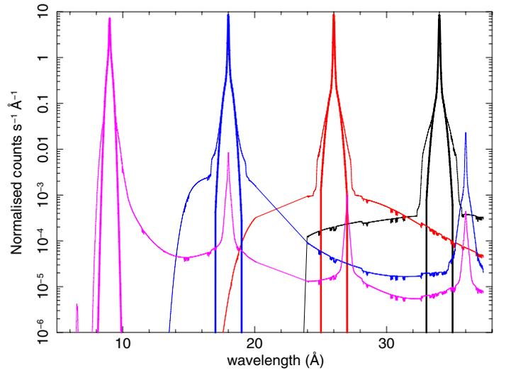
**Fig. 3.** Comparison of the redistribution function for RGS2, first order as delivered by the SAS (thin solid line) to our approximation using three Gaussians (thick lines), for four different photon wavelengths.
