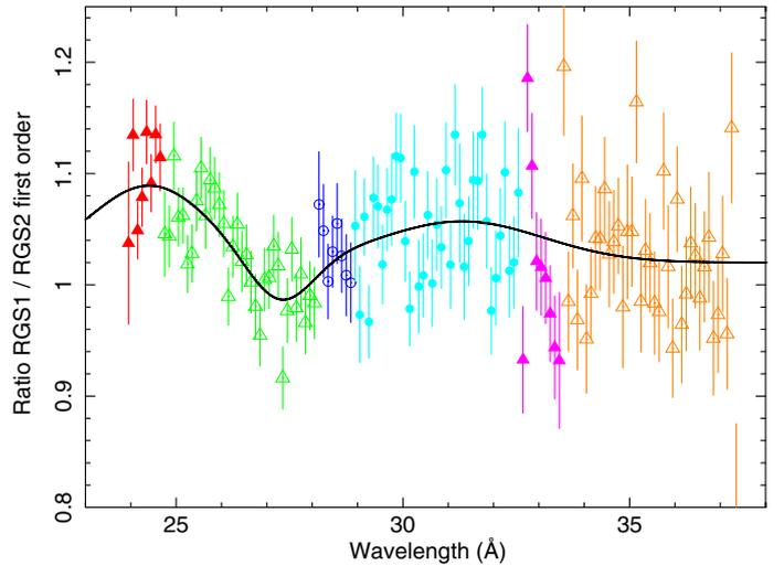
**Fig. 5.** Flux ratio between RGS1 and RGS2 for parts of the spectrum that are detected by both RGS. Different symbols indicate different combinations of CCD chips for both RGS detectors. Open symbols: RGS1 chips 1, 3, 5, 9; filled symbols: RGS1 chips 2, 4, 6, 8. Triangles: RGS2 chips 1, 3, 5, 7, 9; circles: RGS2 chips 2, 6, 8. The solid line is a simple fit to the ratio's using a constant plus Gaussians.
