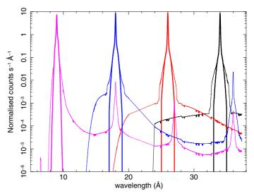
**Fig. 3.** Comparison of the redistribution function for RGS2, first order as delivered by the SAS (thin solid line) to our approximation using three Gaussians (thick lines), for four different photon wavelengths.
