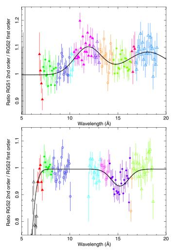
**Fig. 6.** As Fig. 5, but for second-order spectra compared to first-order spectra. Owing to the specific geometry of missing CCDs (CCD7 for RGS1, CCD4 for RGS2) we compare all fluxes to the first order of RGS2. Open symbols: second-order chips 1, 3, 5, 7, 9; filled symbols: second-order chips 2, 4, 6, 8. Triangles: first-order chips 1, 3, 5, 7, 9; circles: first-order chips 2, 6, 8.
