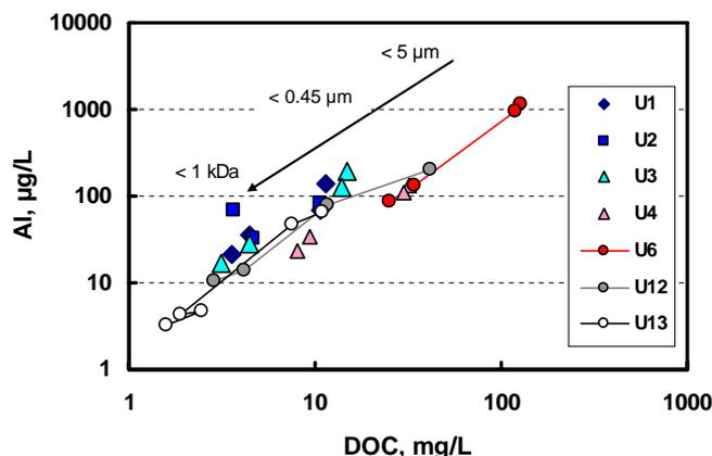
**Fig. 13.** Correlation between Al and DOC in filtrates and dialysates of various samples shown by different symbols (see Table 1 for description). In each series, the first (highest) point corresponds to filtration through 5 or 0.45  $\mu\text{m}$  and the lowest point represents dialysis through 1 kDa.
