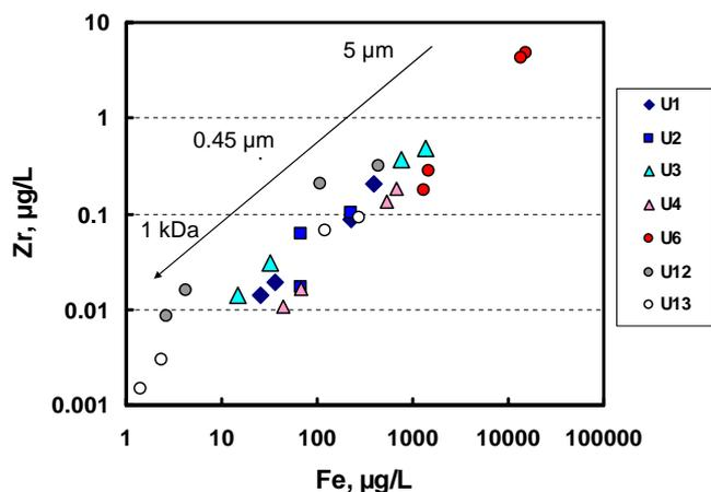
**Fig. 14.** Correlation between Zr and Fe in filtrates and dialysates of various samples shown by different symbols. In each series, the first (highest) point corresponds to filtration through 5 or 0.45  $\mu\text{m}$  and the lowest point represents dialysis through 1 kDa.
