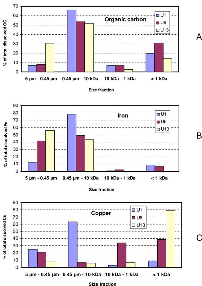
**Fig. 15.** Size fractionation of OC (A), Fe (B) and Cu (C) among main colloidal and subcolloidal fractions in typical samples reflecting three main stages of thaw lake development: U-6, U-1 and U-13 corresponding to peat abrasion, large growing lake and final (khasyrey stage) of the lake.
