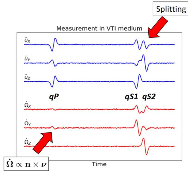
**Figure 1.** Exemplary synthetic six-component borehole seismogram inside a VTI-medium (Taylor Sandstone) with acceleration  $\ddot{\mathbf{u}}$  and rotation rate  $\dot{\mathbf{\Omega}}$  during the arrivals of qP, qS1 and qS2 waves. Two important properties of anisotropic media are evident, namely the splitting of shear waves and the rotation of the qP wave. Portrayed measurements are perturbed with an SNR of 30.
