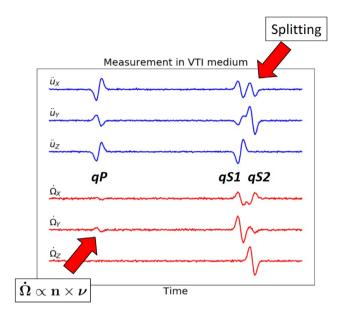
**Figure 1.** Exemplary synthetic six-component borehole seismogram inside a VTI-medium (Taylor Sandstone) with acceleration  $\ddot{\mathbf{u}}$  and rotation rate  $\dot{\Omega}$ during the arrivals of qP, qS1 and qS2 waves. Two important properties of anisotropic media are evident, namely the splitting of shear waves and the rotation of the qP wave. Portrayed measurements are perturbed with an SNR of 30.
