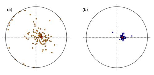
**Figure 9.** Estimated symmetry axis directions from calculated elastic tensors for  $10^{\circ}$ -tilted Taylor Sandstone at an SNR of 100 using (a) rotation method and (b) strain method. True symmetry axis indicated by cross. Vertical direction in the centre and the circle indicates horizontal directions.
