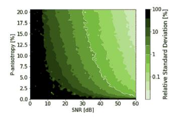
**Figure 5.** Relative standard deviation of rotation-derived *P*-wave velocities with respect to SNR and *P* anisotropy  $(\max_{\theta} v_p(\theta)/\min_{\theta} v_p(\theta) - 1)$  at an angle of incidence of 58°. The synthetic materials have been produced by linearly changing the values of the Thomsen parameters of Taylor Sandstone (Thomsen 1986). The default Taylor Sandstone has a *P* anisotropy of 10 per cent. Standard deviations based on 50 repetitions for each material-SNR pair.
