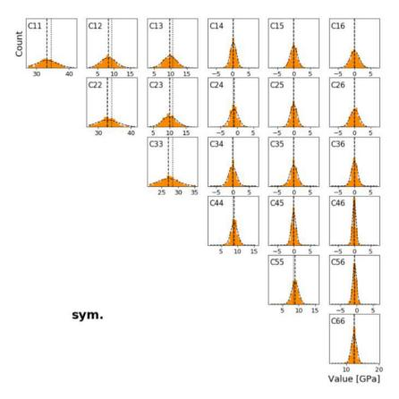
Figure 7. Histograms for 500 repetitions of the elastic tensor inversion at an SNR of 100 in a  $10^{\circ}$ -tilted Taylor Sandstone. The arrangement of histograms mirrors the appearance of the Voigt-notation elastic tensor. True values are indicated by dotted vertical lines. Dashed vertical lines are the mean value of the inversion and the Gaussian curves are maximum-likelihood solutions. The resolution of elastic parameters depends on the location inside the elastic tensor.
