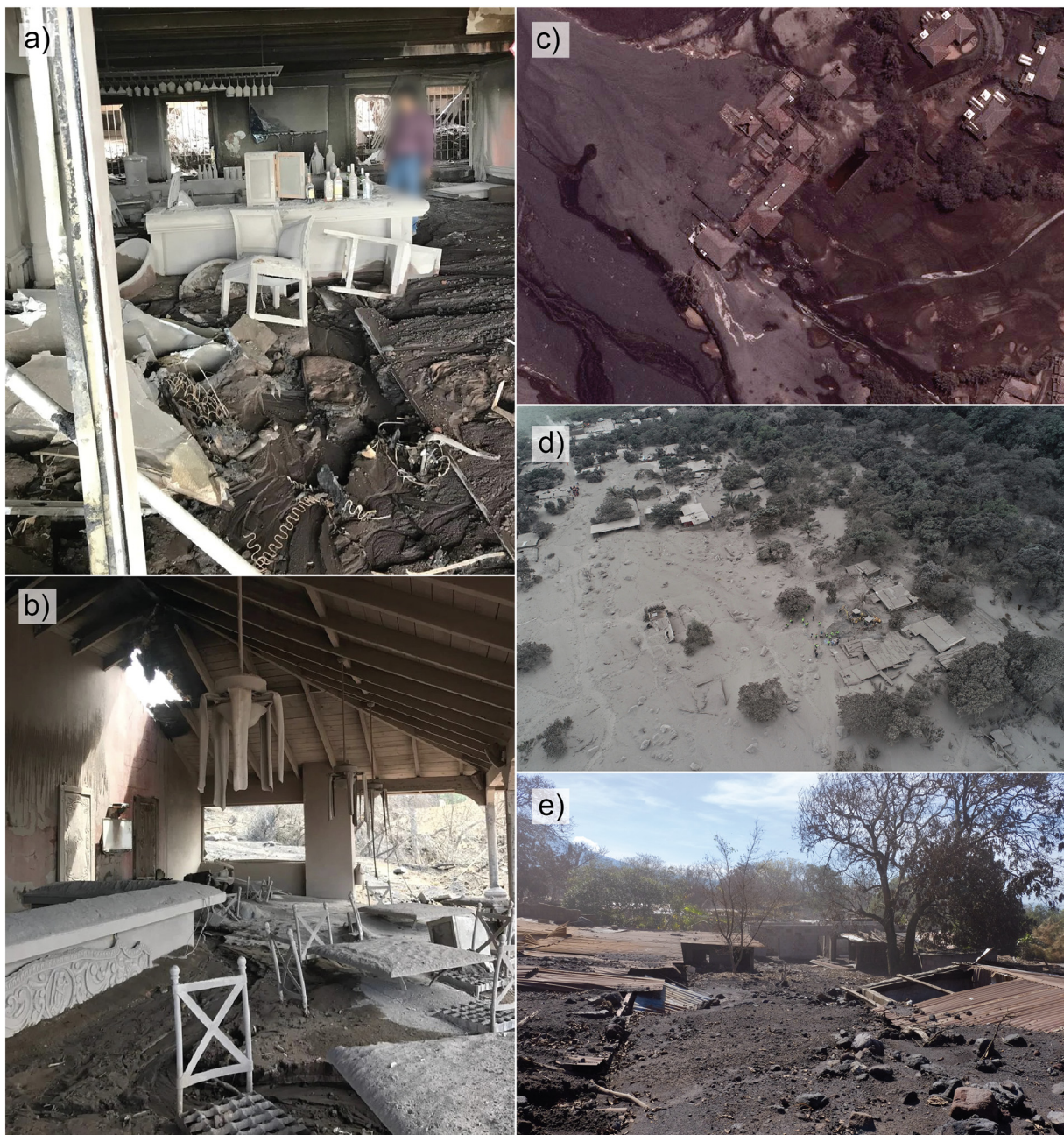
Fig. 9. a) inside of La Reunión clubhouse building showing effect of LEDS (ash-covered bottles on counter) and post-eruption lahars (knocked over chairs) (22 June 2018), b) inside of clubhouse building showing overspill deposits to chair height, LEDS deposits of a few centimetres on tables, isolated fire damage to roof, and ceiling fan melted due to radiant heat from overspill deposits (22 June 2018); c) Digital Globe satellite imagery of La Reunión golf resort (acquired three days after impact on 6 June 2018) showing partially inundated clubhouse building. Different shade of grey between left and right side of the buildings shows deposition areas of dense overspill flows (L) which were stopped by structures and LEDS (R) which were able to flow past (adapted from imagery provided by Maxar Technologies under CC BY-NC 4.0); d) aerial photo of San Miguel Los Lotes, facing south, showing fully destroyed northern end of town (bottom of frame) with large boulders, contrasted with mostly undamaged buildings at the south end of town (top left of frame) (AP, 5 June 2018), e) buried buildings in the town of San Miguel Los Lotes showing minimal structural damage and deposits surrounding and on top of buildings (P. J. Baxter, 25 June 2018).
