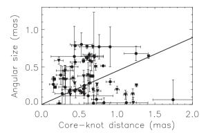
**Figure 6.** Angular size of jet components as a function of their separation from the core at 15, 24 and 43 GHz (circles, upside-down triangles and squares, respectively). Linear regression of the data (solid line) leads to an apparent jet opening angle of  $24^{\circ}.1 \pm 0^{\circ}.3$ .
