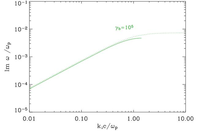
**Figure 3.** Same as Fig. 2, but for the filamentation instability. The calculation assumes  $k_{\parallel} = 0$ . Only the growth rate for  $\gamma_b = 10^5$  is shown, as smaller values of  $\gamma_b$  did not lead to exact growing solutions.
