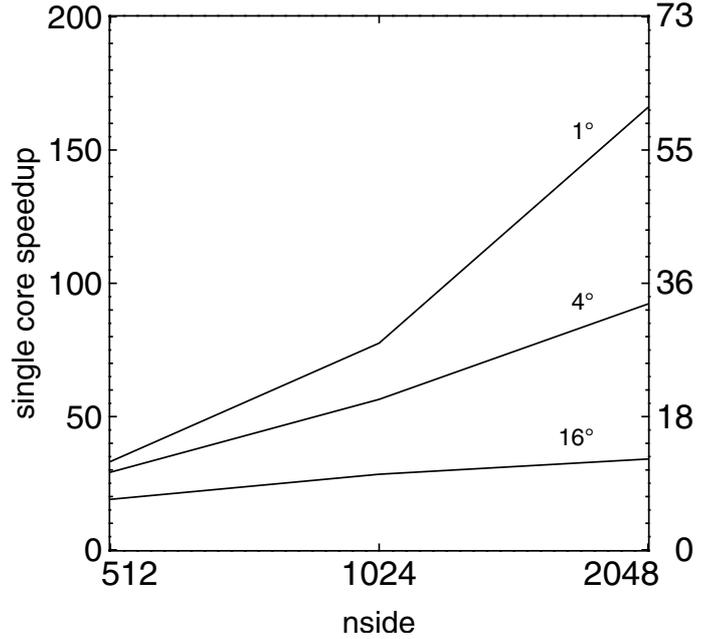
**Fig. 2.** Performance gain of the GPU-based convolution code when compared to the HEALPix FSHT-based implementation (left axis) and the `libpsht` library (right axis) running on a single CPU core for different map resolution parameters and kernel support.
