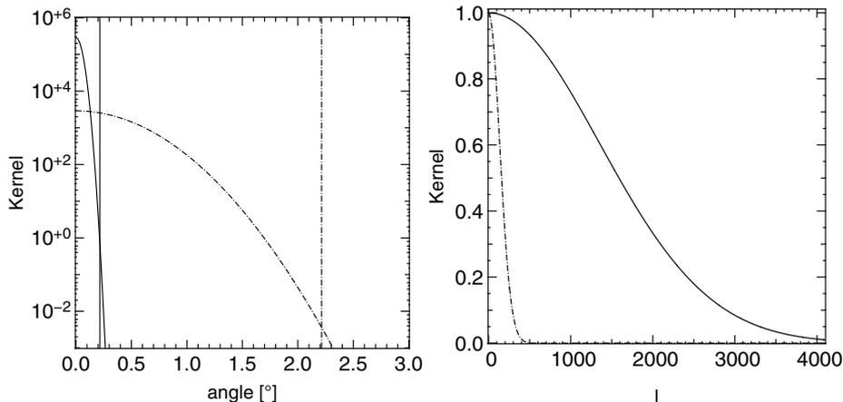
**Fig. 3.** Profile of the kernels used for our accuracy tests. *Left panel:* we show the pixel space representation of a Gaussian kernel with  $6'$  (solid line) and  $1^\circ$  FWHM (dashed line). The vertical lines indicate the angle beyond which the kernel is truncated. *Right panel:* legendre expansion of the kernels (solid line:  $6'$  FWHM, dashed line:  $1^\circ$  FWHM). Kernels that are compact in pixel space cover a wide range of modes in spherical harmonic space and vice versa.
