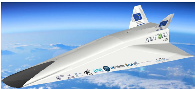
Fig. 2 STRATOFLY MR3 external configuration
