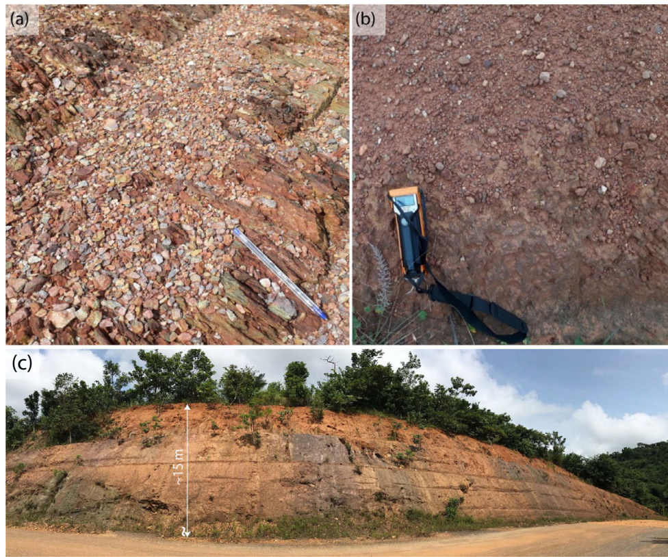
Fig. 8. Images of K-poor areas: (a) weathered metasedimentary rock (saprock) exposed on the surface, outcrop BO39 ( 6^{\circ}32.25'N/1^{\circ}21.35'W ), 14 cm pen for scale. b) Lateritic cover outside of the outer ring anomaly, outcrop BO29 ( 6^{\circ}29.10'N/1^{\circ}31.33'W ), portable gamma-ray spectrometer RS-230-BGO (26 cm long) for scale. c) Outcrop at location BO34 ( 6^{\circ}25.47'N/1^{\circ}25.9'W ), outside the ejecta deposits and, therefore, beyond the outer ridge. Here, a thick lateritic cover is exposed in a road cut. This about 15 m thick lateritic cover is likely representative of the subsurface in the area surrounding the impact structure. The locations of these outcrops are indicated in Fig. 2. (Color figure can be viewed at wileyonlinelibrary.com .)
