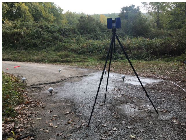
Fig. 1 This tiny scarp on the La Rouvière tar road was the first evidence of Le Teil earthquake-related ground rupture uncovered by the field team (2 days after the event). The equipment is a laser scanner to image accurately the offset.
