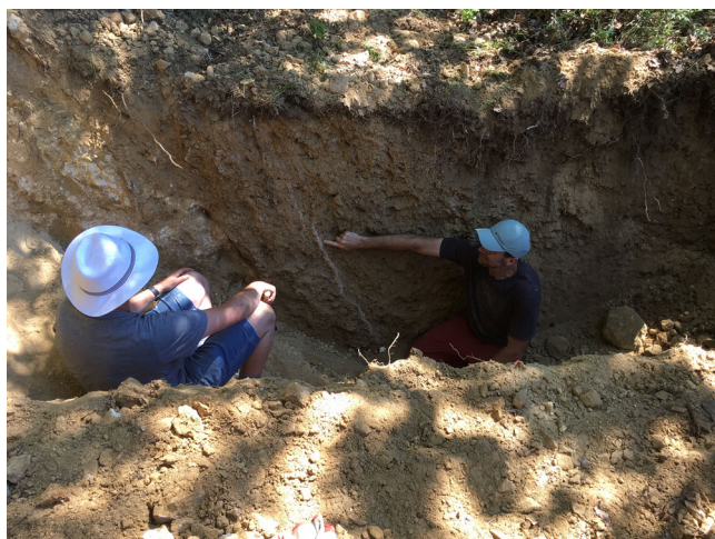
Fig. 2 Detail picture of a trench wall excavated across the causative fault. This is from the first trench out of a dozen that was dug during the 2020 spring; notice the fracture in the colluvium related to a pre-historical activity, with the two authors for scale.
