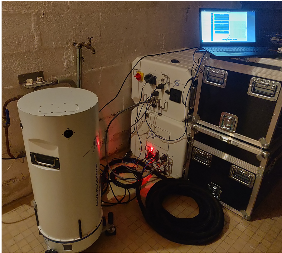
Figure 1. AQG-B01 in a garage in Montpellier in June 2020. The sensor head (left) is connected with the laser and electronic systems by 5 m of cables. The AQG GUI software is used on a laptop to control the measurement as well as to correct, visualize, and analyse the gravity data.
