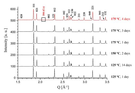
**Figure A11.** XRD measurements of experimentally altered *Arctica islandica* samples subjected to alteration temperatures between 125 and 175 °C for various lengths of time (1, 2, 3, 4 and 14 days). Calcite formation starts at 175 °C and an alteration time of 4 days. Miller indices for calcite (Cc) are given in red and those for aragonite in black.
