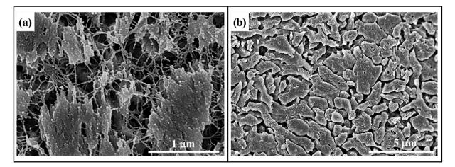
**Figure A8.** Pristine (**a**) and hydrothermally altered (**b**) shell portion of *Arctica islandica*. Alteration occurred in burial fluid at  $175 \,^{\circ}$ C and lasted for 7 days. Well visible in (**a**) is the network of biopolymer fibrils between and within pristine aragonite nanoparticles and mineral units. This is destroyed at alteration and numerous voids (**b**) become visible within the mineral units.
