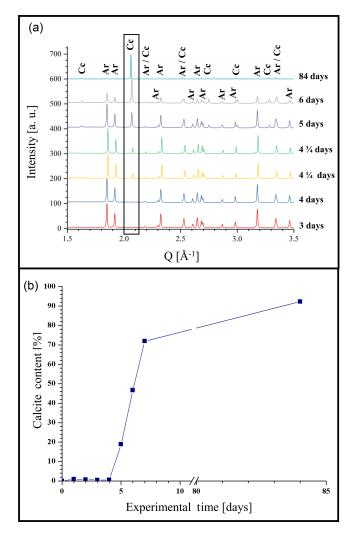
**Figure 8. (a)** Selected X-ray diffractograms for 3 to 84 days of alteration of *Arctica islandica* shell material. Alteration took place in artificial burial solution at 175 °C. (b) Newly formed calcite content relative to alteration time (days) calculated from Rietveld analyses of the XRD measurements.
