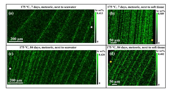
**Figure A6.**  $Sr^{2+}$  concentrations along annual growth lines in hydrothermally altered *Arctica islandica* shell portions. Alteration temperature was 175 °C, meteoric water was used as alteration fluid, and the alteration experiments lasted for 7 and 84 days (**a–b**).  $Sr^{2+}$  concentration scatters for both alteration times around 0.4 wt %  $Sr^{2+}$  and is similar to the value measured in the pristine *Arctica islandica* reference samples (see Fig. A5a, b).
