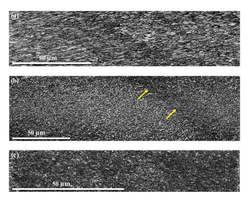
**Figure A9.** EBSD band contrast images taken along a cross section from different parts of the shell of pristine *Arctica islandica*. (a) Outer shell layer, (b) central shell section, and (c) inner shell layer. Well visible is the difference in crystallite size. In contrast to the outer shell layer (a), the innermost shell section is highly dense and consists of minute aragonite crystals.
