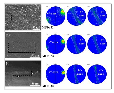
**Figure A10.** Pole figures obtained from EBSD measurements shown in Fig. A9. Measurements are performed on pristine *Arctica islandica*. SEM images on the left-hand side indicate the location of EBSD maps: (a) outer shell layer, (b) central shell portion, (c) inner shell layer. The pole figures and MUD values indicate clearly that aragonite co-orientation increases significantly towards innermost shell sections.
