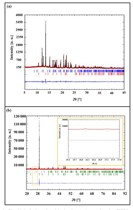
**Figure A12.** Representative Rietveld plot for the product of the alteration experiment performed at 175 °C for 6 (a) and 84 days (b) in artificial burial solution measured with  $MoK_{\alpha 1}$  in transmission and with  $CuK_{\alpha 1}$  in reflection, respectively. The diffuse amorphous signal peaking near 12.5° 2 $\theta$  is due to the Lindemann glass capillary ( $\emptyset$  0.3 mm) containing the sample.
