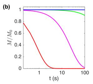
**Figure 1.** (a) Variations of relaxation time with diameter of spherical magnetite-like minerals and (b) corresponding magnetization decay normalized by initial magnetization  $M_0$ . Blocking volume with stable magnetization (blue), thermally active particles with viscous (green and magenta) and fast (red) magnetic relaxation as expected in 100 s window.
