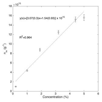
**Figure 6.** SPCDM estimates for particle concentration versus true mass concentration.
