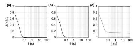
Figure 3. Magnetization relaxation after applying a 500 mT normalized by in field magnetization  $M_0$ ; (a) nanoparticle of synthetic magnetite with fast relaxation; (b) air particulate matter with same behaviour and (c) sediments from Jaraguá Cave with slower magnetization decay, suggestive of coarser SP minerals
