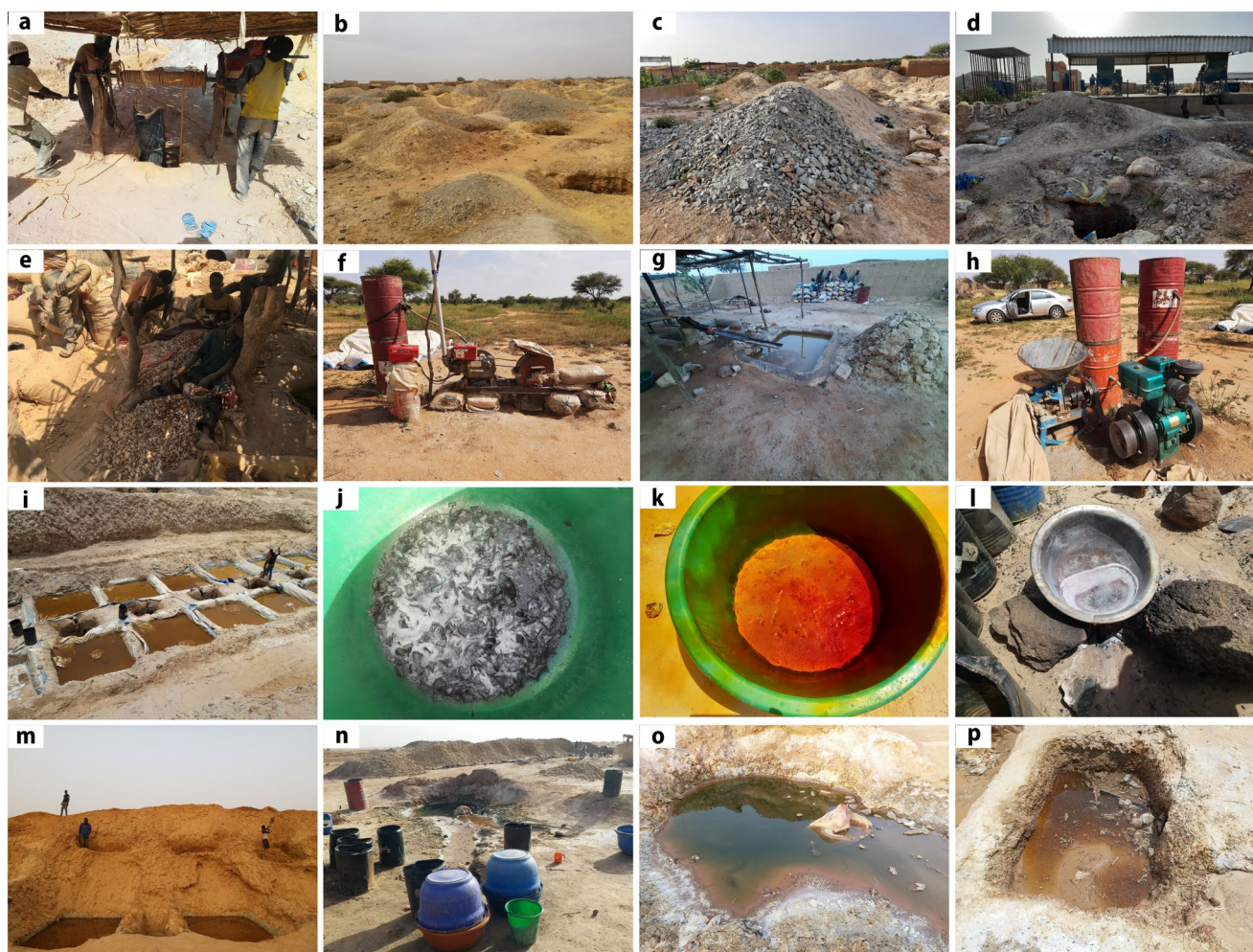
Figure 3. The Koma Bangou gold panning waste production: (a) workers operating a hoist on a gold mining pit; (b) clay minerals-rich tailings around dwellings; (c) quartz diorite tailings near houses; (d) ore extraction pit with crushing machines just behind; (e) manual crushing of gold-bearing quartz; (f) quartz ore fragments crushing machine; (g) gravimetric concentration of gold by sluice; (h) grinding machine for the fine residues from the gravimetric concentration; (i) alignment of cyanidation ponds; solution of gold-bearing zinc with nitric acid (j) and sulfuric acid (k); (l) gold concentration by firing with nitric acid and sulfuric acid; (m) pile of cyanidation solid waste; (n) place of acid treatment of gold; (o) acidic liquid residue from the chemical treatment of gold; (p) storage hole for acidic liquid waste.
