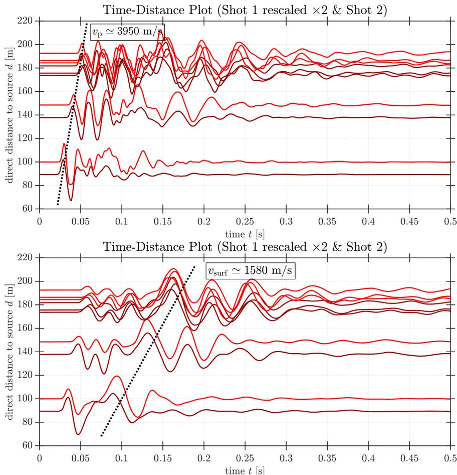
**Figure 3.** Time–distance plots of the vertical ground velocity normalized in amplitude. Data are bandpass filtered in the 0.5–1000 Hz range on top, and in the 0.5–20 Hz range at the bottom. The distance  $d$  is the direct distance to the explosive charges, in meters.  $v_p$  and  $v_{surf}$  stand, respectively, for  $P$ - and surface wave velocities.
