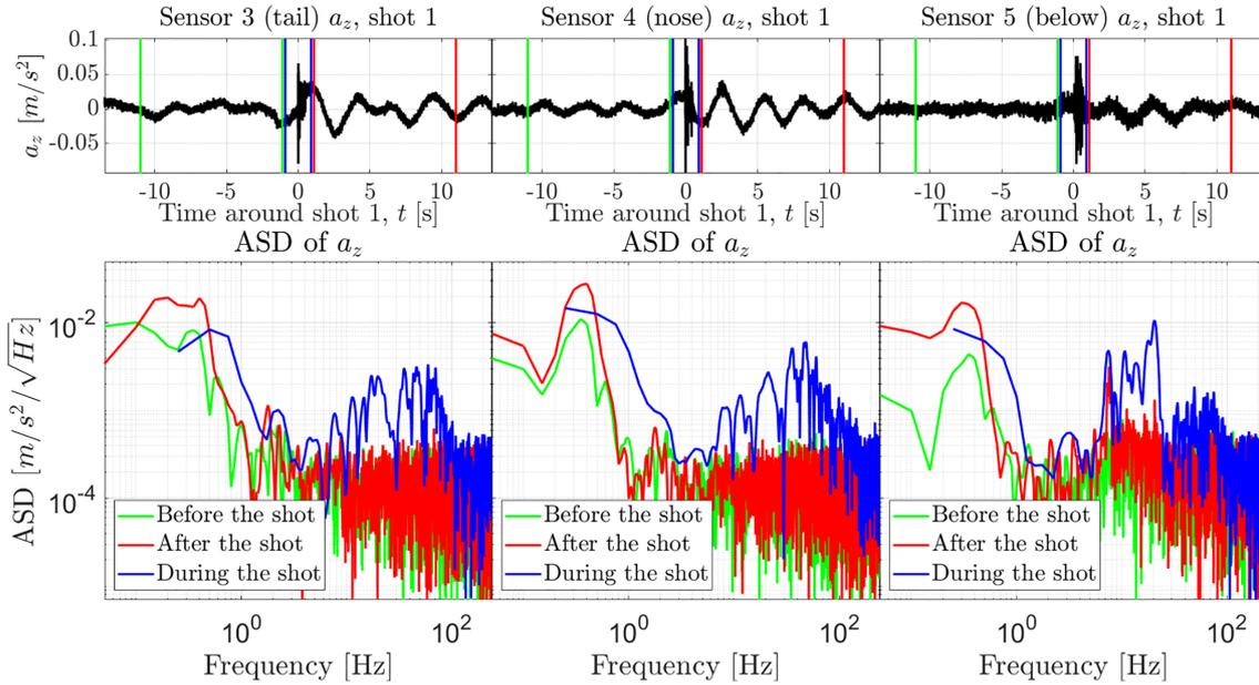
**Figure 7.** ASD of the vertical acceleration (de-trended) of the three sensors in the balloon referential, around shot 1. The ASD are plotted with different windows of time represented by the coloured lines. The ASD exhibit the tethered-balloon resonance modes below 1 Hz, as well as the infrasonic signals in the 10–30 Hz frequency range during the shot.
