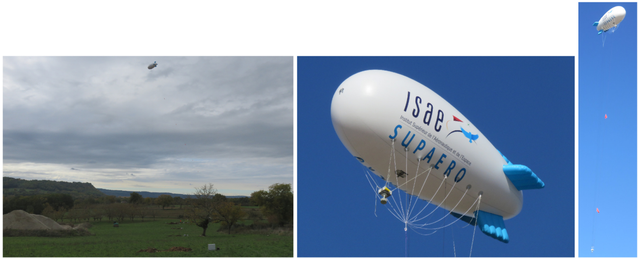
Figure 2. Left: picture taken from shot zone and looking towards the ground instrument line (marked by holes in the ground) and balloon deployment. Middle: balloon, showing upper infrasound sensor and two IMUs taped on envelope at the nose and the bottom of the balloon. Right: balloon and tethering system, showing the two identical infrasound sensors attached to the balloon platform. One at the bottom of the image (40 m below the balloon) and one attached just below the balloon (better seen in the middle image).
