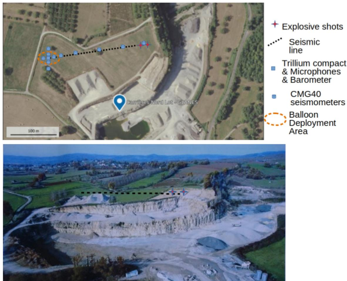
**Figure 1.** On the top: view from the top of the experiment setup indicating the positions of the shots, the various sensors and the balloon location. On the bottom: aerial view of quarry showing the shots location and the topography.
