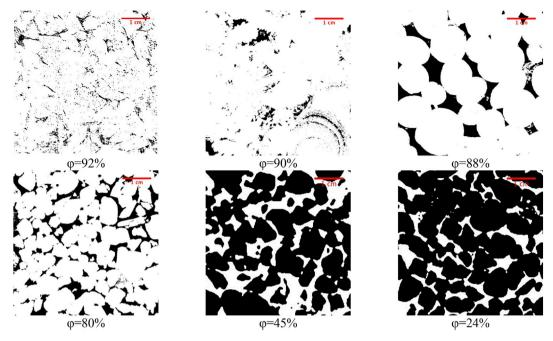
Fig. 1. Binary X-Ray Micro-CT image cross section of porous medium samples used with a resolution of  $5 \mu m$ . White colour is porous material and black colour is void area.
