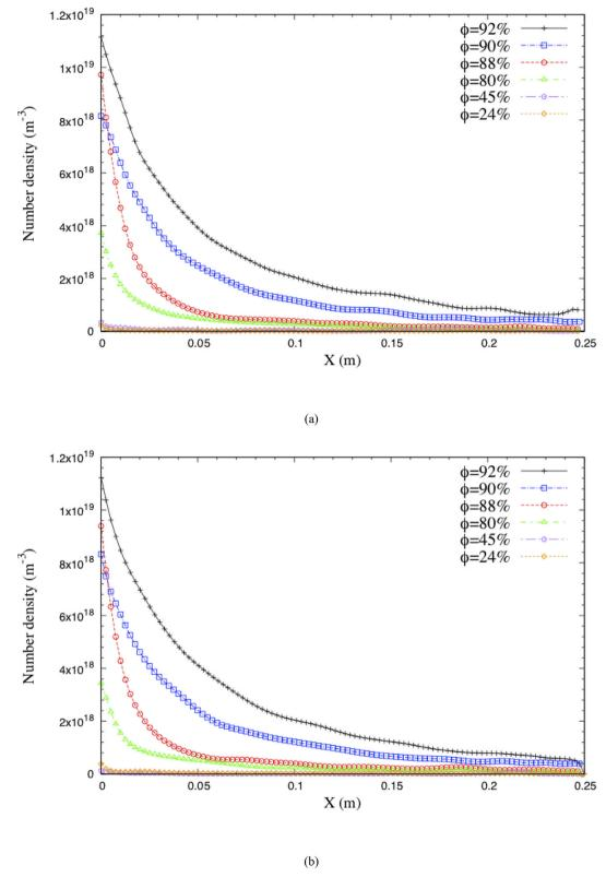
Fig. 7. Outgassing number density profiles above the surface as function of porosity based on rock temperature, 300K (a) and 330K (b).
