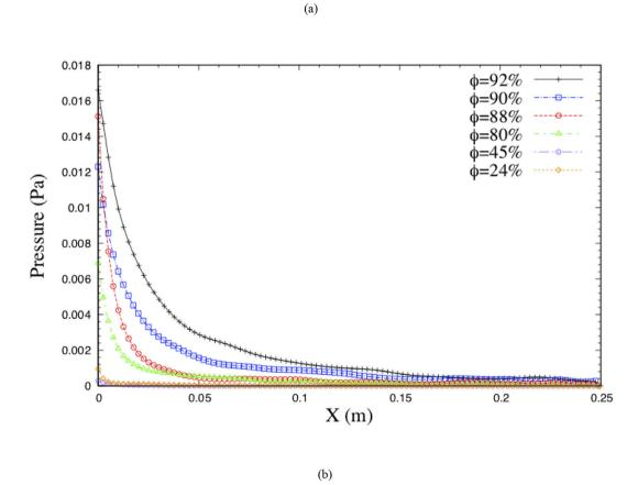
$\textbf{Fig. 5.} \ \ \textbf{Outgassing gas pressure as function of porosity for two porous medium temperatures, 300K (a) and 330K (b). \\$
