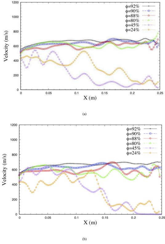
Fig. 8. Outgassing velocity profiles above the surface in a range of porosities for rock temperature a) T = 300K and b) T = 330K.
