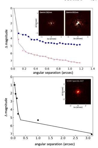
**Figure 7.** Contrast curves showing the  $5\sigma$  detection sensitivity and speckle autocorrelation functions. The top panel shows the data obtained using Zorro on Gemini with the filters centred on 562 nm (blue squares) and 832 nm (red crosses) and the bottom panel shows the observations obtained with the HRCam speckle imager on SOAR in the *I*-filter.
