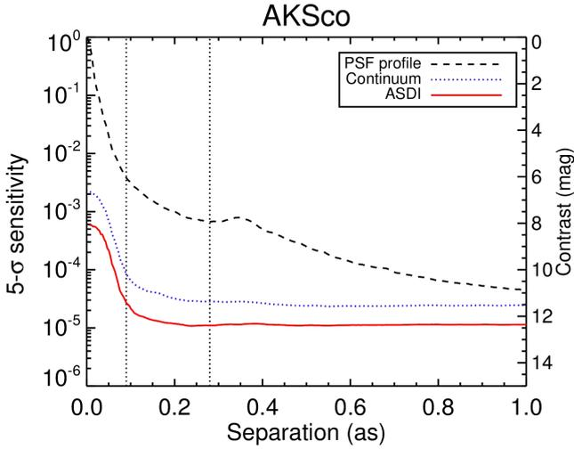
**Fig. 3.** Contrast plot for the object AK Sco. In a black solid line, the profile of the PSF is shown, blue represents the H $\alpha$  continuum filter after being processed with PCA and ADI, and red is the ASDI contrast. The vertical dotted lines represent the extension of the spirals (Janson et al. 2016).
