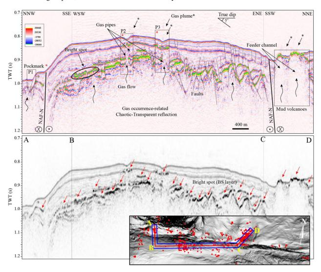
**Fig. 8. a**: Multichannel seismic response of the mud volcanoes "yellow line in B". White star-the mud volcano which is the closest to the NAF-N; Black star- the next mud volcano; Yellow star-the buried mud volcano. **b**: Time slice at 1.0 s "red line in A". Mud structures area shown by yellow dashed polygon without any strata reflectivity. **c1-c2**: Borders of the mud volcanoes below the seafloor (not to scale). They rise up through the seafloor.
