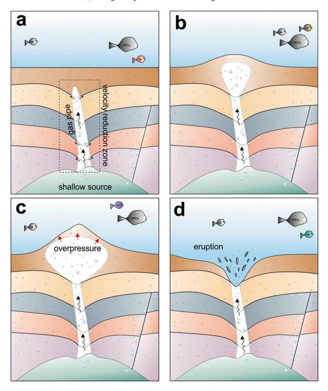
**Fig. 11.** Schematic relationship between the NAF-N and the formation of the mud volcanoes, as well as, gas conduit systems in the Western High. Thermogenic gas migrates from source/reservoir rock via the NAF-N and mud volcanoes to shallow depth. (ps: illustration is not to scale).
