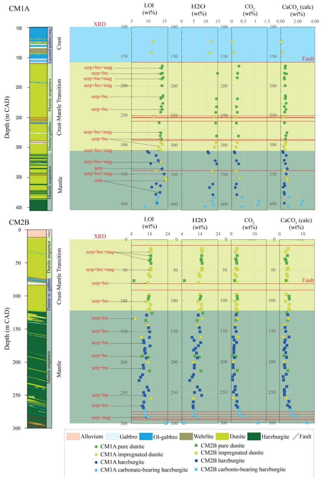
**Figure 3.** Downhole plots of (from left to right) the lithology, loss on ignition (wt.%), H<sub>2</sub>O (wt.%), CO<sub>2</sub> (wt.%) and calculated CaCO<sub>3</sub> (wt.%) contents in pure dunites, impregnated dunites, harzburgites and carbonate-bearing harzburgites recovered samples at Holes CM1A and CM2B. The thick solid red lines indicate the faults. X-Ray Diffraction, serpentine, brucite, magnetite.
