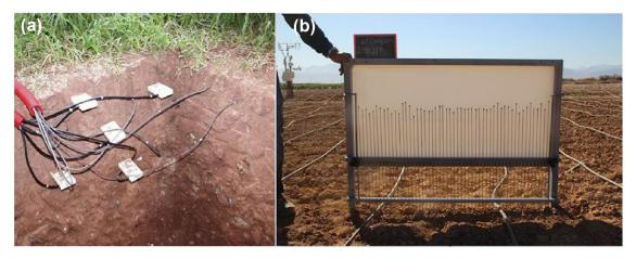
Figure 2. Examples of (a) TDR sensors installed at different depths and (b) a pin profiler picture taken over one of the plowed field with drip irrigation tubes installed.
