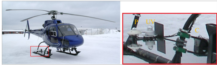
Figure 1. Pyranometer (P), UV sensor (UV) and camera (C) attachment to the helicopter. The other pairs of pyranometers and UV sensors are attached to the opposite landing gear symmetrically. The thermometer and the humidity sensor are attached at the back of the opposite landing gear below the fuselage.
