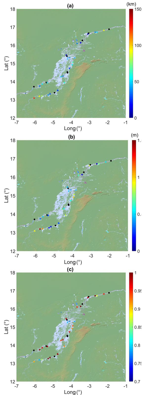
**Figure 3.** Comparisons between in-situ and altimetry-based water levels for Sentinel-3A (upward-pointing triangles) and 3B (downward-pointing triangles) over the IND: (a) distance between in-situ stations and VS, (b) RMSE (m), (c)  $R$ .
