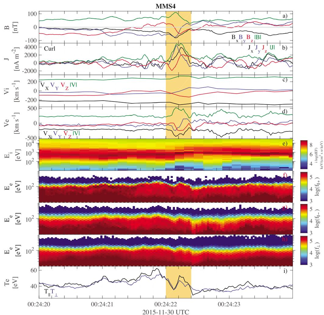
**Figure 3.** Overview of the current sheet. Unless otherwise stated, all coordinates are in GSE. (a) The magnetic field; (b) current; (c) ion velocity; (d) electron velocity; (e) ion omnidirectional fluxes; (f–h) parallel, antiparallel, and perpendicular electron distribution; and (i) parallel and perpendicular electron temperature. The orange shaded area indicates the studied current sheet.
