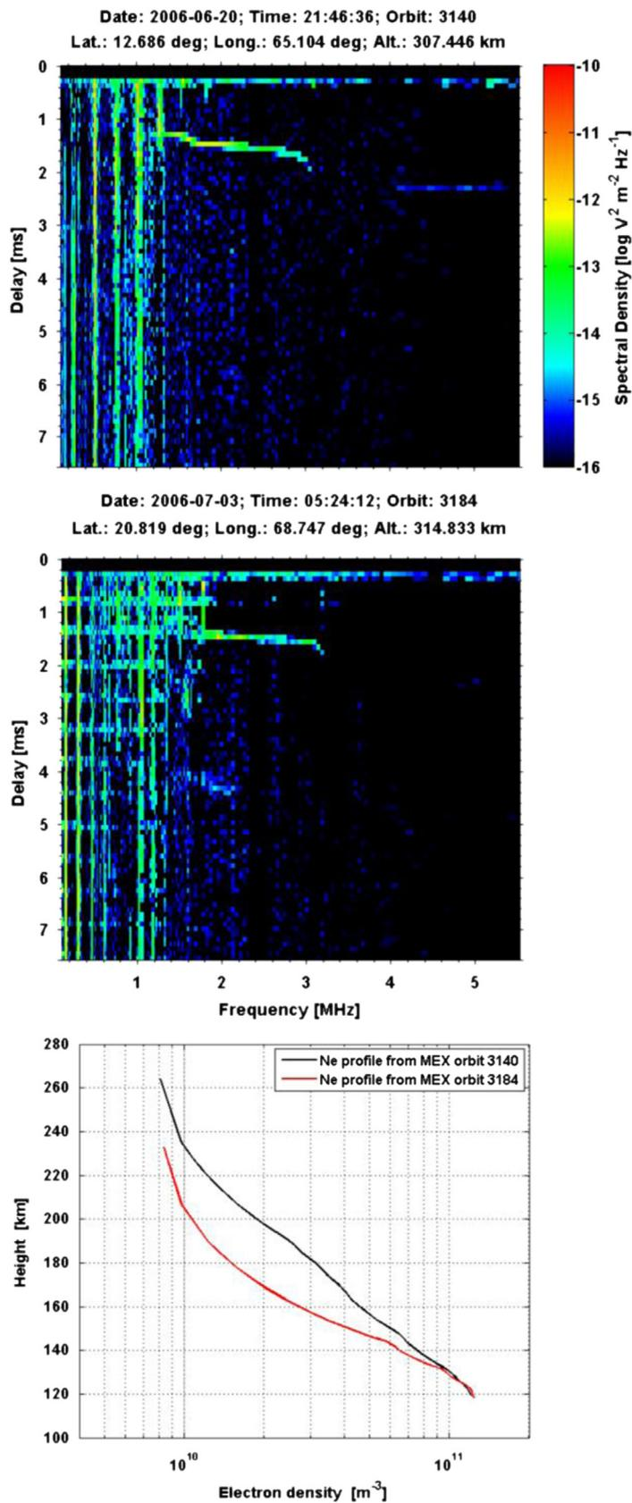
**Fig. 4.** Example of ionograms from the pericenter of the orbit for when there is not magnetic field at the spacecraft location (upper panel) and for when there is magnetic field (medium panel). Both ionograms belong to the orbits of Fig. 3. The horizontal echoes of the second case are caused in last instance due to the presence of a magnetic field at the spacecraft surroundings. In the bottom panel, two typical electron density profiles from these orbits.
