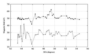
**Fig. 9.** Magnitude of magnetic field measured by MARSIS in orbit 3151 at the spacecraft position (black dotted-line) and magnitude of the magnetic field at the transition altitude derived from the pressure balance (white dotted-line) for the same orbit, versus solar zenith angle.
