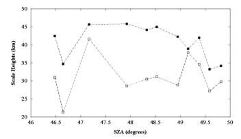
**Fig. 8.** Mars Express Orbit 3151: values of the two plasma scale heights found in the profiles, as a function of solar zenith angle. Black squares: plasma scale height of the photochemical-controlled region (region in the profile close to the peak). White squares: plasma scale height of the region under the influence of the magnetic field penetration (diffusive region, top part of the profile).
