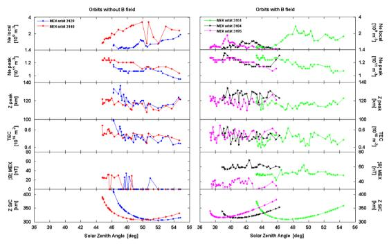
**Fig. 5.** Solar zenith angle series of the main characteristics of the 5 Mars Express orbits of this study. The panels of the figures show from the top to the bottom: local and peak electron densities, peak altitude, total electron content of the topside ionosphere, magnitude of the magnetic field measured by MARSIS and spacecraft altitude. Note that all the panels have the same scale at each orbit, except the MARSIS magnetic field one.
