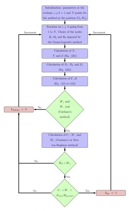
Fig. 2. Algorithm to determine the value, 0 or 1, of the function 1 ballistic according to the initial conditions. Once this value is known, we use Eq. (24).
