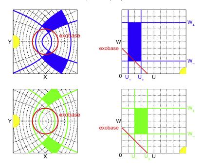
**Fig. 1.** Representations of areas where ballistic (blue) and satellite (green) particles evolve in the usual coordinate system (left panel) and in the (U,W) plane. To pass from the left grid to the right one, we apply the transformation  $(x,y) \rightarrow \left(u = \sqrt{x^2 + y^2} + x, \ w = \sqrt{x^2 + y^2} - x\right)$ . (For interpretation of the references to color in this figure legend, the reader is referred to the web version of this article.)
