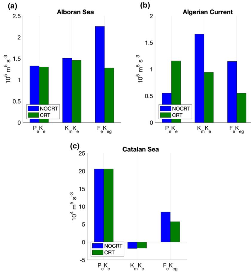
**Figure 7.** Depth-integrated simplified EKE-budget components based on a temporal Reynolds decomposition ( $\text{m}^5 \text{s}^{-3}$ ) from NOCRT (blue) and CRT (green) over (a) the Alboran Sea, (b) the Algerian Current, and (c) the Catalan Sea. The eddy wind work ( $F_e K_{eg}$ ) is positive due to the presence of wind-driven currents along the coast.
