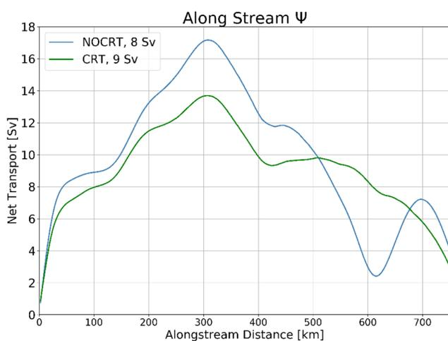
**Figure 11.**  $\Psi$  along the Algerian Current (see Figure 3), from NOCRT and CRT. On the one hand, CFB slows down the Algerian Current from NOCRT to CRT by 10% on average but up to 20%. On the other hand, in NOCRT, standing eddies near Sardinia causes a strong disruption of the Algerian Current, largely reducing the net transport. CFB, by damping these eddies, stabilizes this part of the Algerian Current. CFB, current feedBack to the atmosphere.
