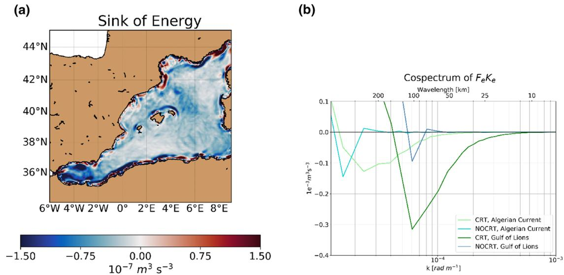
**Figure 8.** Exchange of energy between oceanic mesoscale currents and the atmosphere. (a) Spatial distribution of the eddy wind work estimated from CRT using a spatial filter, allowing to filter out most of the wind-driven currents. (b) Co-spectrum of  $F_e K_e$  over the Algerian Current and the Gulf of Lions (see boxes on Figure 1) from NOCRT (blue) and CRT (green). CFB causes sinks of energy from oceanic mesoscale currents to the atmosphere. CFB, current feedback to the atmosphere.
