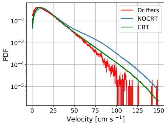
**Figure 6.** Probability density function of surface current velocity from drifters (red), NOCRT (blue), and CRT (green). The surface currents from the simulations have been smoothed using a two-day window to be comparable to drifters estimate. The error bar is estimated as the square root of the count of each bin. The number of bins (150) is estimated based on Freedman and Diaconis (1981).
