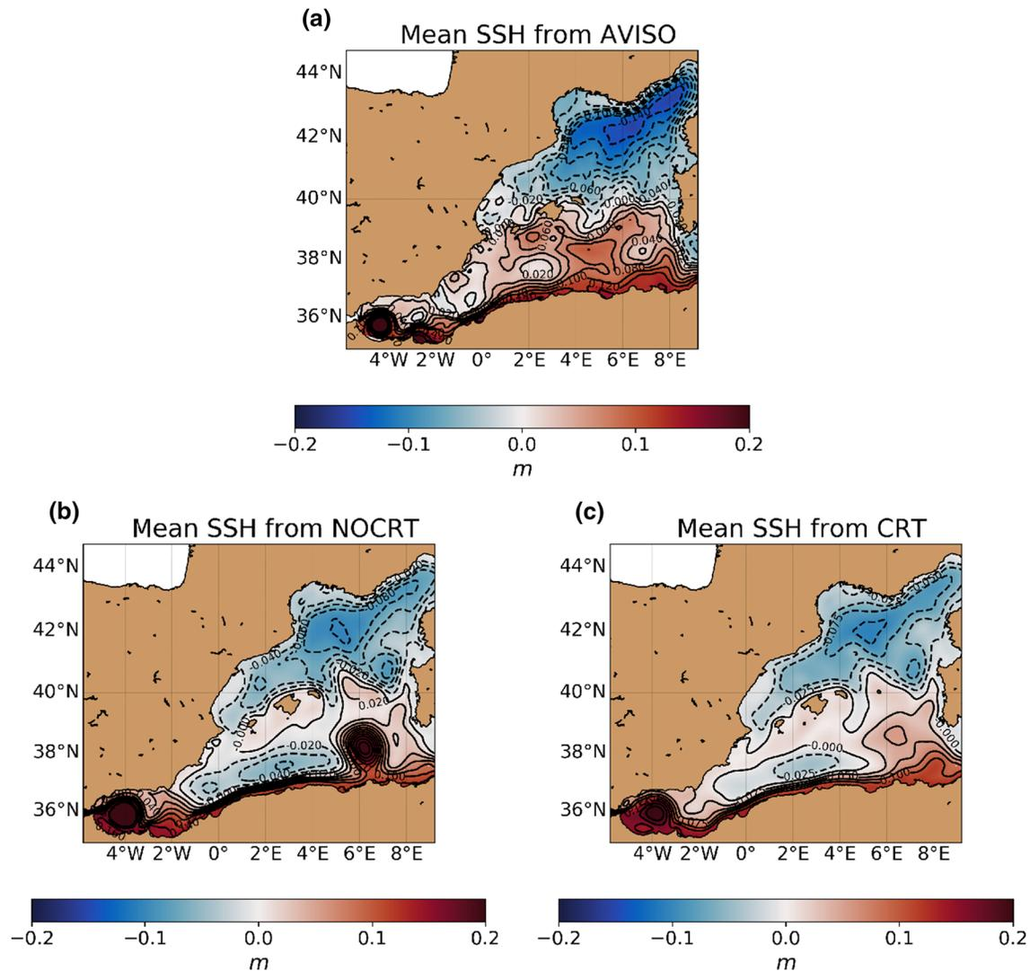
**Figure 2.** Mean sea surface height (SSH) from (a) the AVISO product, (b) the simulation without CFB (NOCRT), and (c) the simulation with CFB (CRT). CFB, current feedback to the atmosphere. AVISO, Archiving, Validation and Interpretation of Satellite Oceanographic data.
