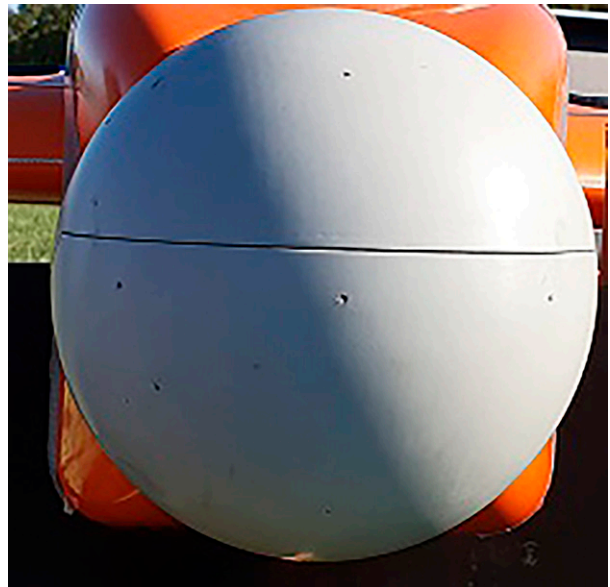
FIG. 3. Picture (front view) of the five-hole probe mounted on BOREAL.
