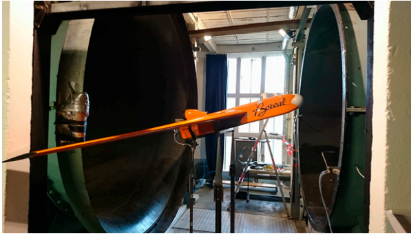
FIG. 11. BOREAL in the wind tunnel test at IMFT.
